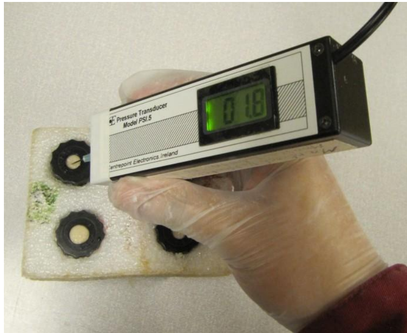
Fig. 8 Measuring the pressure in SAA test.
