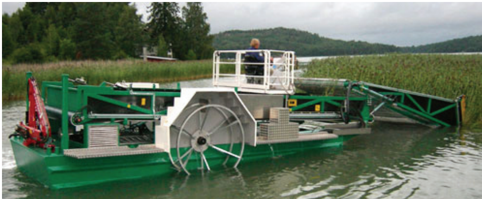
Figure 1.5. Aquatic Plant Harvester RS 2000 (From RS-Planering AB, 2008).
