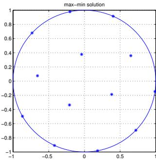
(b) Local optimal solution from solving the Max-min optimization problem for  $n=13$  using a random initial estimate. The values of the maximum minimal distance and the potential are:  $Min - dist = 0.6090$ ,  $Pot = 78.2893$
