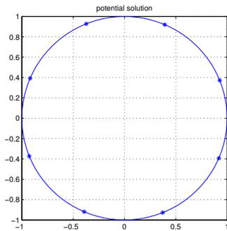
(a) Global Optimal solution from solving the Potential optimization problem for  $n=8$  using a random initial estimate. The values of the maximum minimal distance and the potential are:  $Min - dist = 0.7651$ ,  $Pot = 22.4389$
