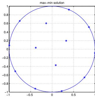
(a) Global optimal solution from solving the Max-min optimization problem for  $n=13$  using a random initial estimate. The values of the maximum minimal distance and the potential are:  $Min - dist = 0.6180$ ,  $Pot = 76.7786$
