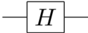
Figure 2.2: Circuit representation of the Hadamard gate. [8]
