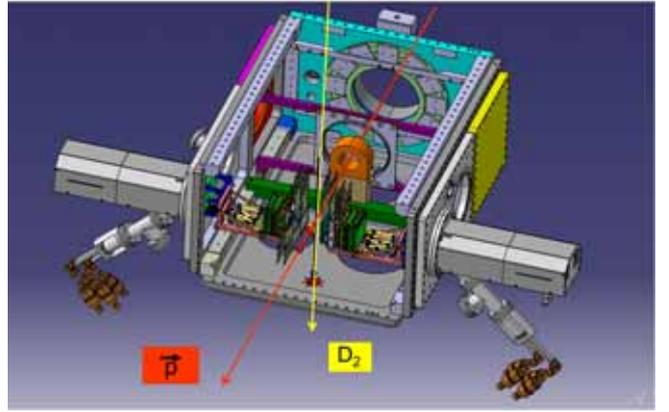
Figure 3: Experimental setup for the measurement of the beam polarization. The cluster target beam comes from the top and traverses the beam stored in the machine. Recoil deuterons are detected by two Silicon Tracking Telescopes (STTs) left and right to the beam.
