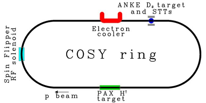
Figure 1: Schematic view of the COSY storage ring. The polarized hydrogen target is installed in one of the straight sections of the ring; the RF solenoid of the Spin-Flipper is located in one of the arcs, its use is explained in more detail in the text; the Electron Cooler, followed by the detector setup with Silicon Tracking Telescopes (STTs) to determine the beam polarization, is installed in the second straight section.
