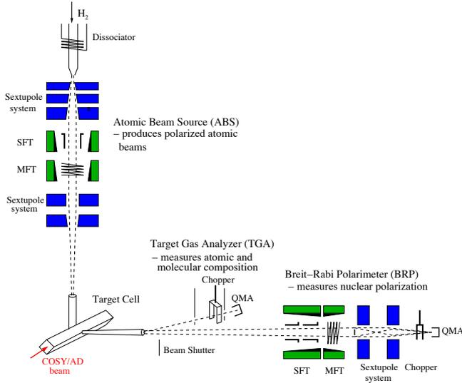
Figure 2: Schematic drawing of the PAX polarized target with the ABS in the vertical position, the storage cell on the ring axis, and the target diagnostic system in the horizontal position. The Target Gas Analyzer (TGA) determines the atomic to molecular fraction of the effusive beam from the storage cell, while the Breit-Rabi Polarimeter (BRP) measures the degree of polarization of the atomic sample.
