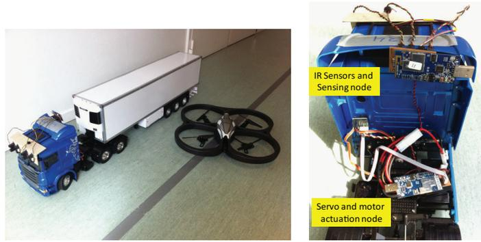
(a) ARdrone Quadrotor and Heavy-Duty Vehicle (b) Heavy-Duty Vehicle with Telosb nodes
