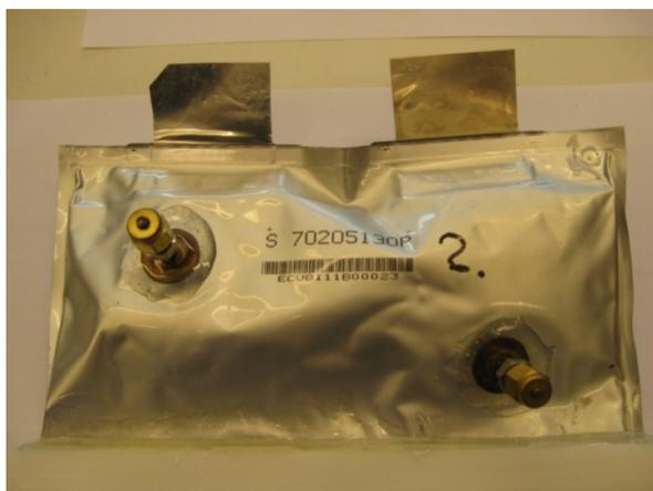
Water vapour transmission measurements were performed according to the standard test method for water vapour transmission rate through plastic films and sheeting, ASTM F 1249-05 [14]. Preconditioning of the packages was carried out in an environment where the humidity was close to 0%. Temperature and relative humidity (RH) measurements inside the plastic box that was acting as a
