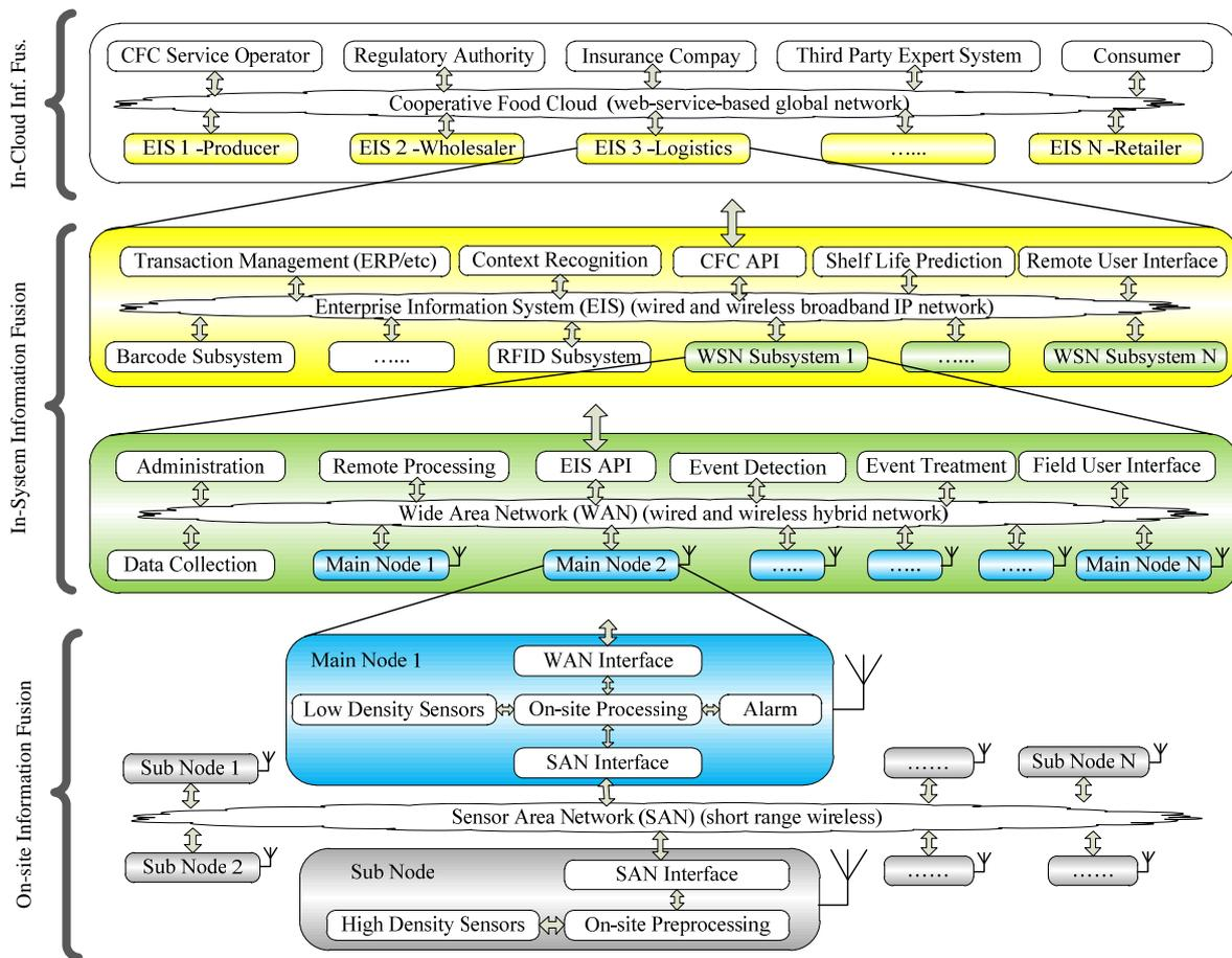
Figure 3-1 A hierarchical EIS architecture of the proposed Food-IoT solution
