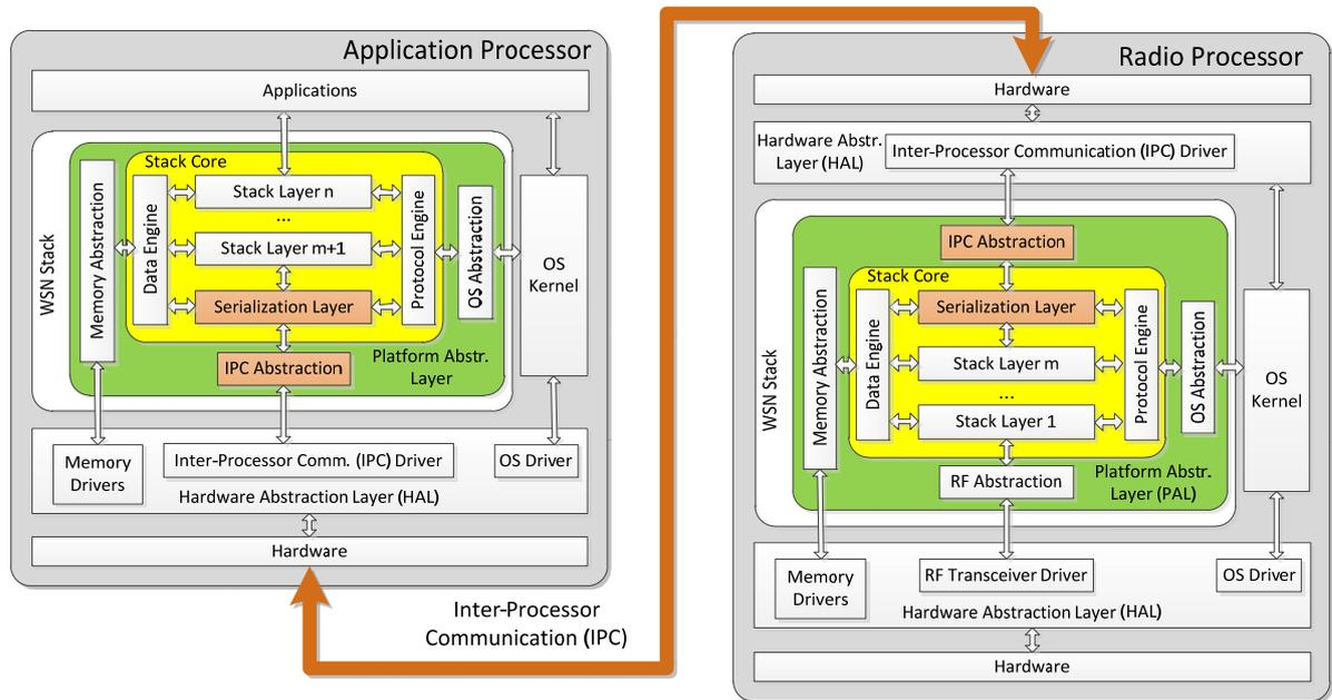
Figure 2-2 The proposed RTOS-based WSN stack architecture with multiprocessor support
