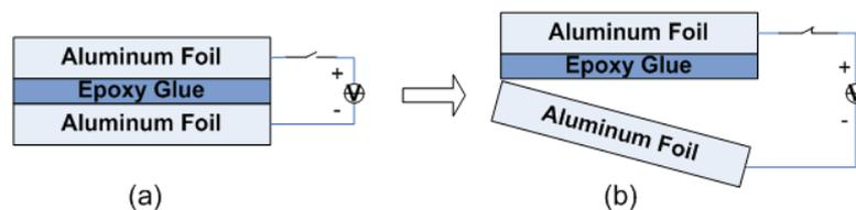
Figure 2-5 Illustrated structure and delaminating behavior of the CDM
