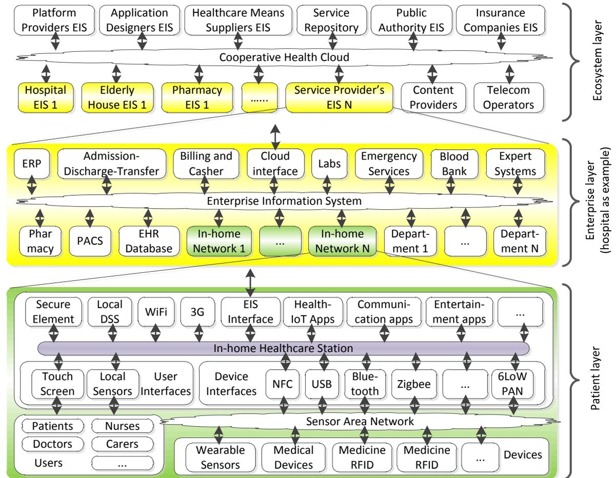
Figure 3-2 A hierarchical EIS architecture of the proposed Health-IoT solution
