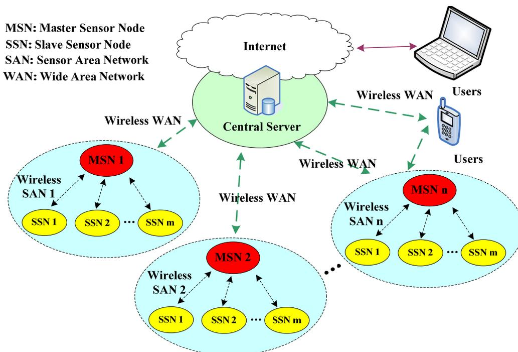
Figure 2-1 The proposed WAN-SAN Coherent Architecture of WSN
