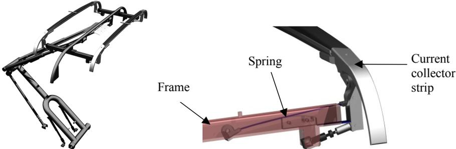
Figure 3. A Schunk WBL88X2 pantograph and its current collector strip suspension [8].
