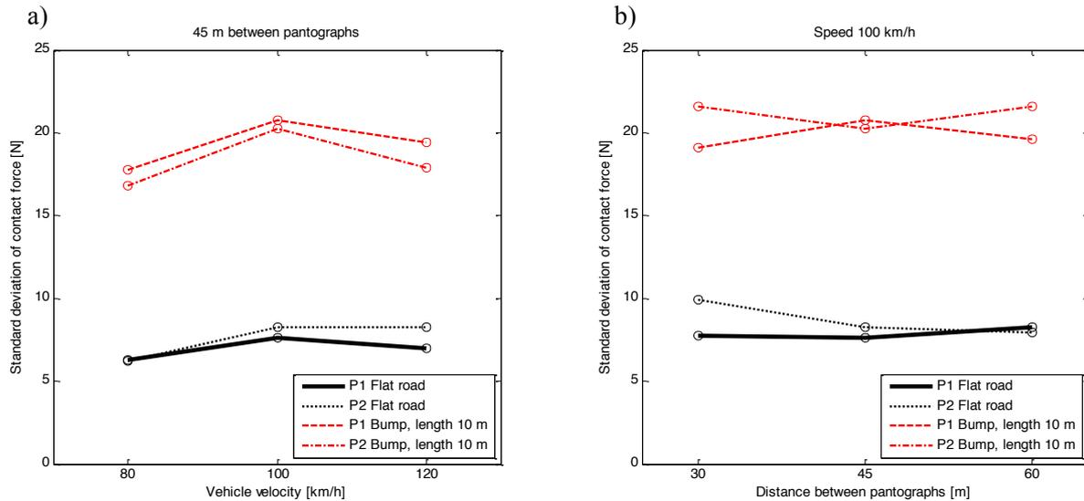
**Figure 8. a)** The contact force standard deviation as a function of speed for a pantograph distance of 45 m. The results are for flat road and a road with a 10 m long bump at a support pole. **b)** The contact force standard deviation as a function of pantograph distance at a speed of 100 km/h. The results are for flat road and a road with a 10 m long bump at a support pole.
