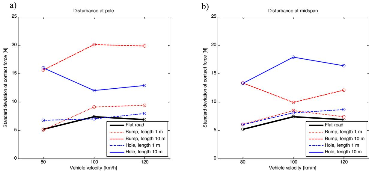
**Figure 7.** The contact force standard deviation as a function speed for **a)** flat road and road irregularities introduced at the support pole and **b)** flat road and road irregularities introduced at the midspan.
