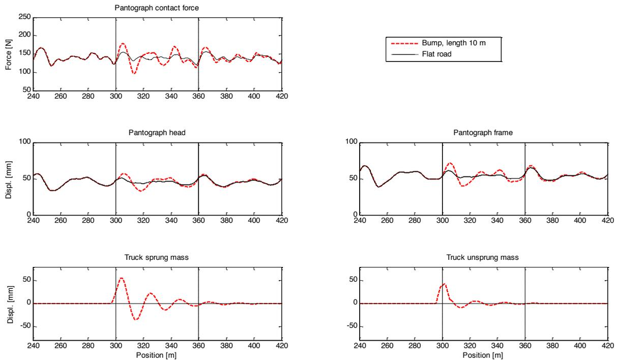
**Figure 6.** Pantograph contact force, pantograph displacements and truck displacements as a function of position along the catenary when a truck is running at 100 km/h. Solid line represents running on a flat road and dashed line represents when running on a road with a 10 m long bump at the support pole.
