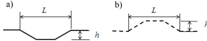
**Figure 5.** Illustration of studied road irregularities, **a)** hole and **b)** bump. The length  $L$  is divided into three equally long sections and the amplitude of the disturbance is  $h$ .
