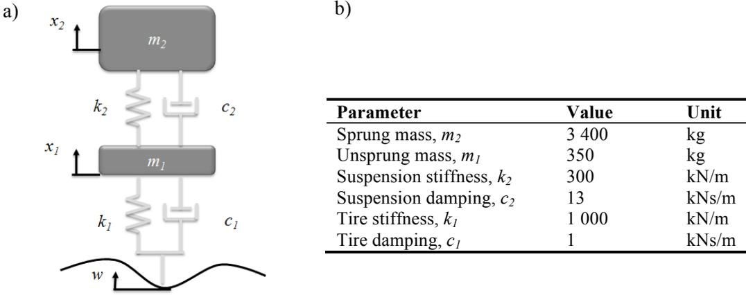
Figure 2. a) The two degree of freedom truck model with road excitation  $w$  and b) the parameter settings for the truck model.
