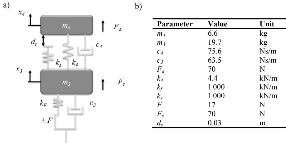
Figure 4. a) The two degree of freedom pantograph model and b) the parameter settings for the pantograph Schunk WBL88X2.
