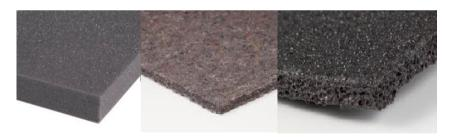
Figure 2.1: Three examples of sound absorbing material: a porous plastic foam, a fibrous lumped material and a metal foam.
