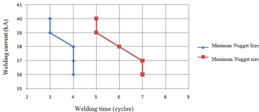
**Figure 7.** The acceptable size of the weld nugget
