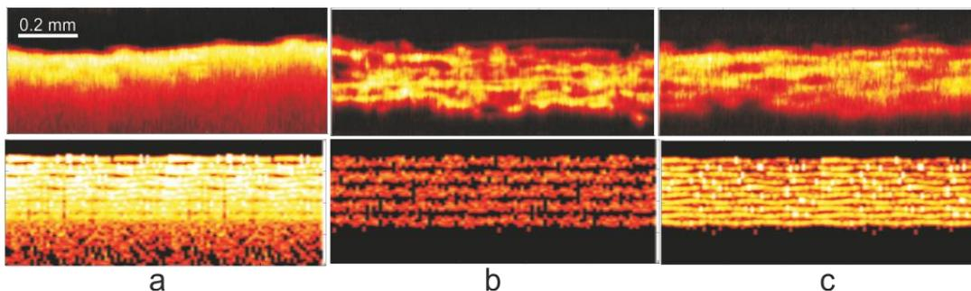
Fig.1. Experimental (top) and simulated (bottom) OCT images of paper samples without optical clearing agent (a), with benzyl alcohol (b), with isopropanol (c).
