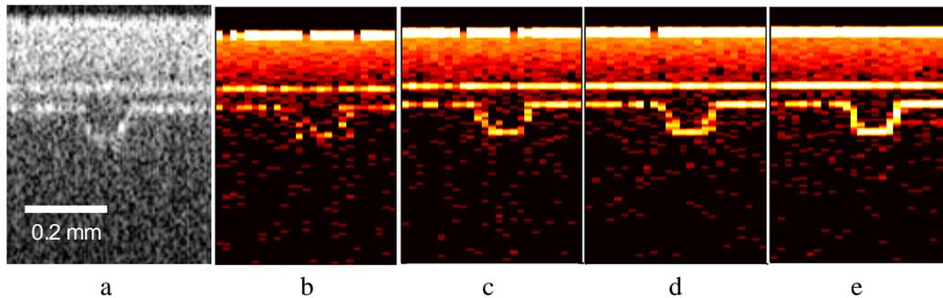
Fig. 2. Experimental (a) and simulated (b-e) cross-sectional OCT images of the stacked alumina layers with embedded microchannel for different RMS roughness of the surface: (b) 140 nm, (c) 90 nm, (d) 60 nm, (e) 30 nm.
