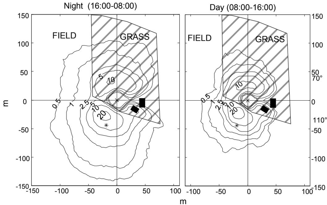
Figure 4: Integration of source areas (%) in the eddy-correlation measurements for night-time fluxes (left) and daytime fluxes (right), 1998-08-18 to 1999-07-29. The position of the soil profile measurements (\*), the observatory buildings (filled rectangles) and the border between grassland (shaded area) and agricultural fields are indicated in the graphs.
