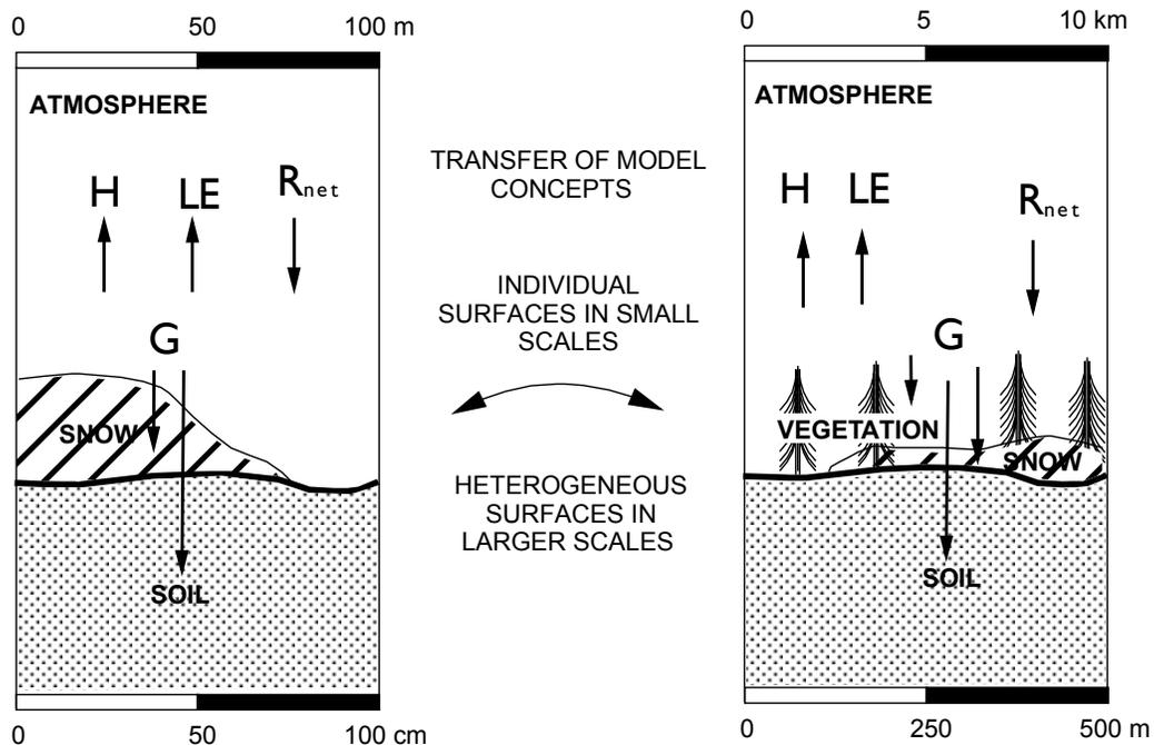
Figure 1: Conceptual view of the heat balance in the soil-snow-(vegetation)-atmosphere system at two approximate scales of measurements and models considered in the present study (arrows signify the positive sign). Symbols refer to eq. (1) below.
