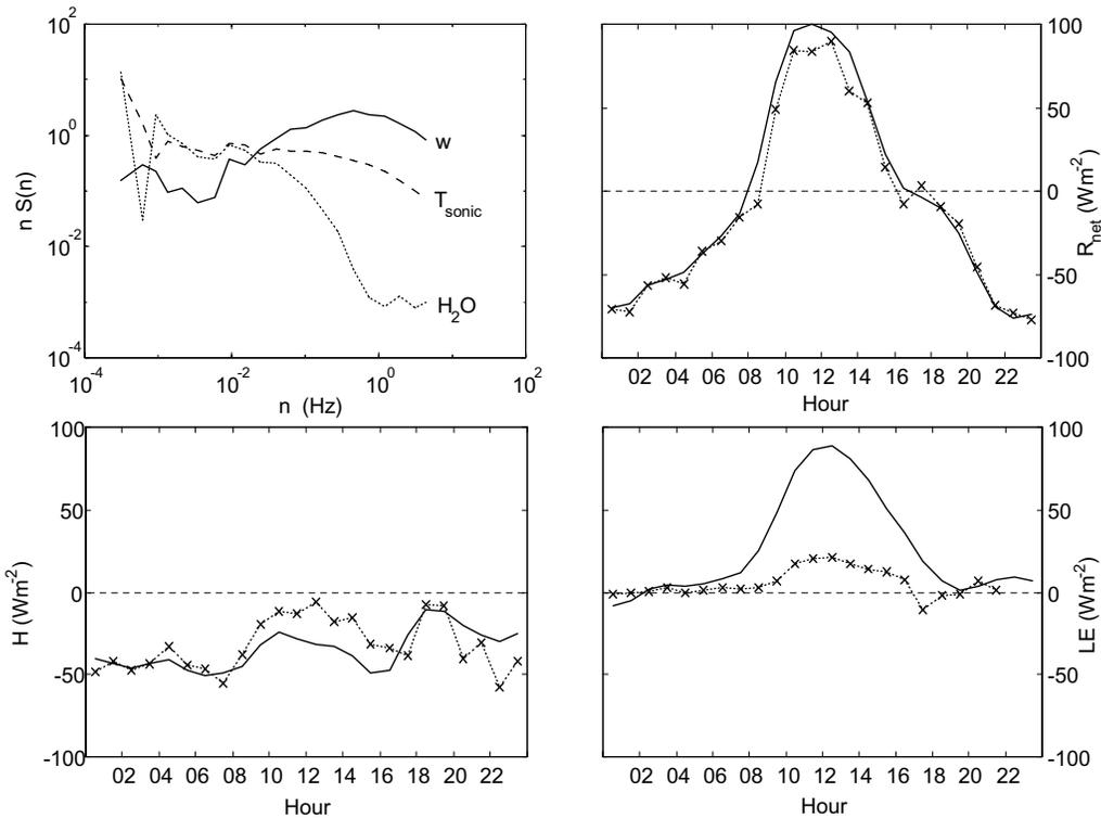
Figure 5 (a): power spectra from the eddy-flux station estimated from 23 February 1998, showing an unrealistic frequency loss in the water-vapour signal compared to vertical wind-speed and sonic temperature signals. (b-d): net radiation loss from the grassland (dashed line with markers) and sensible and latent heat fluxes from the eddy-flux station compared with the Coup Model estimates (solid).
