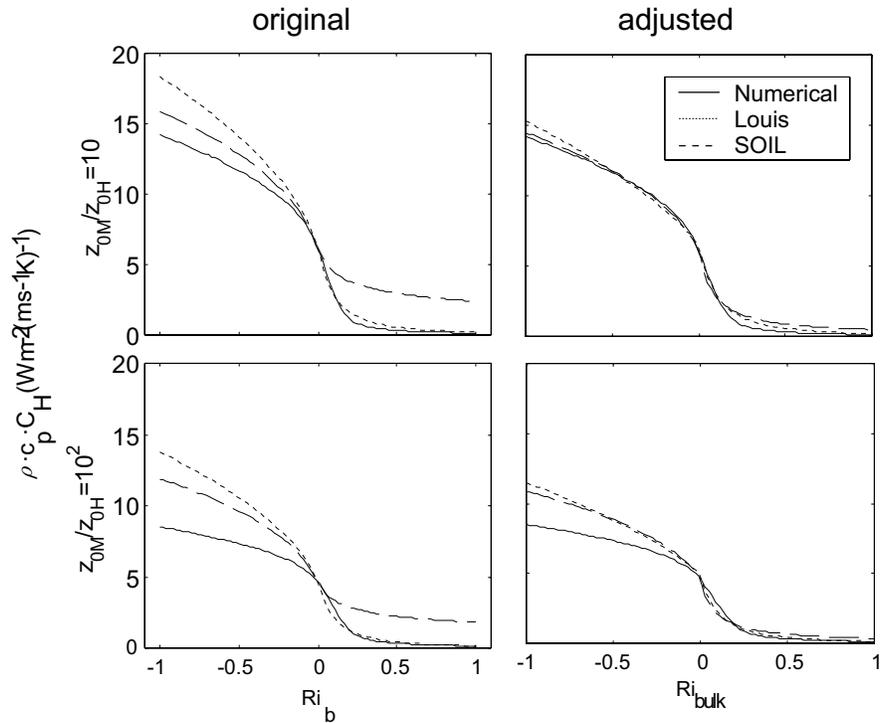
Figure 3: Exchange coefficients for heat derived from empirically found stability functions ("Numerical") and analytical approximations ("Louis" and "SOIL") for  $z/z_{0M}=10^2$  and  $z_{0M}/z_{0H}=10$  and  $10^2$ ; *left*: original parameter values from Louis (1979) and Jansson (1998); *right*: the analytical formulations have been calibrated to the empirically derived exchange coefficients for  $z_{0M}/z_{0H}=10$ .
