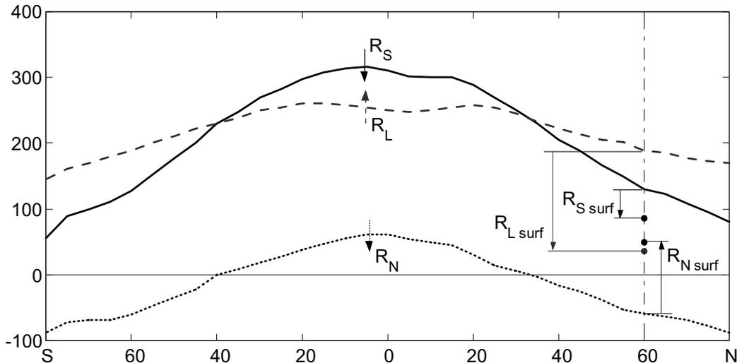
Figure 2: Absorbed solar radiation ( $R_S$ ), outgoing terrestrial radiation ( $R_L$ ) and net radiation ( $R_N$ ) above the atmosphere as function of latitude (after Graedel and Crutzen, 1993) and the net short-wave radiation ( $R_{S\ surf}$ ), net long-wave radiation ( $R_{L\ surf}$ ) and the net radiation ( $R_{N\ surf}$ ) below the atmosphere at Marsta Meteorological Observatory 60°N, Uppsala, Sweden (Halldin et al, 1999) 1998-1999.
