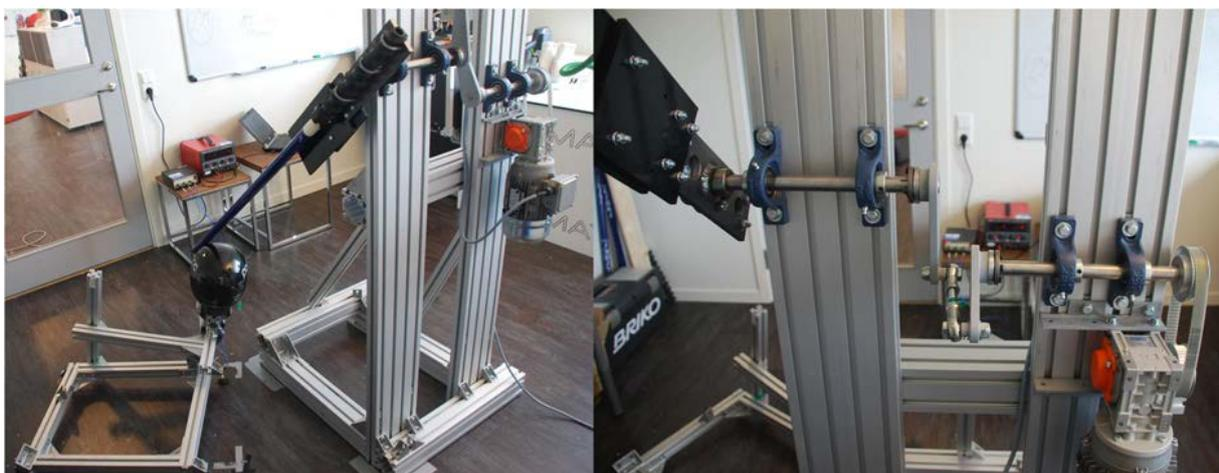
Figure 1. To the left, the test device and the used test setup where the rotating pole impacted the helmet on the left side of the centerline. To the right, a close-up on the drive chain with the motor in bottom right corner and with the attached gearbox which drives the two drive shafts that are connected with asymmetrical mounted rods.
