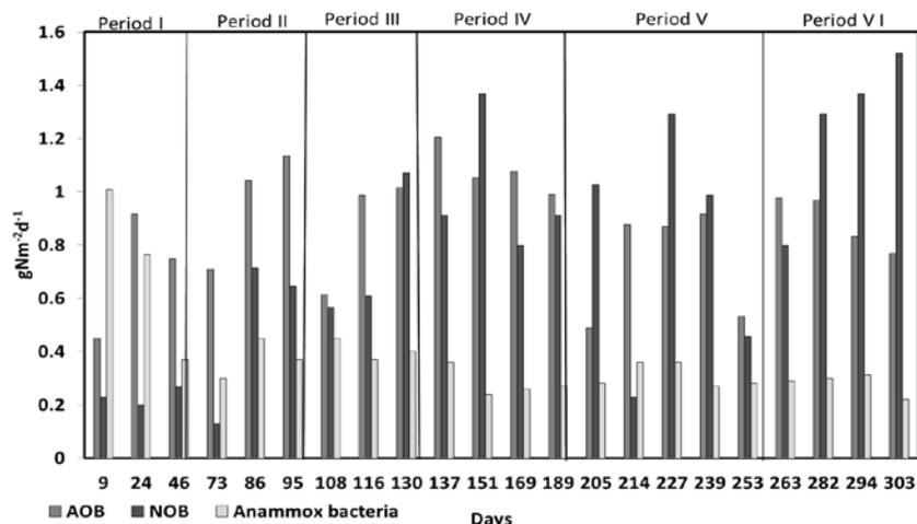
**Fig. 11: Nitrogen flux estimation for AOB, NOB and anammox bacteria based on the potential measured by activity tests.**
