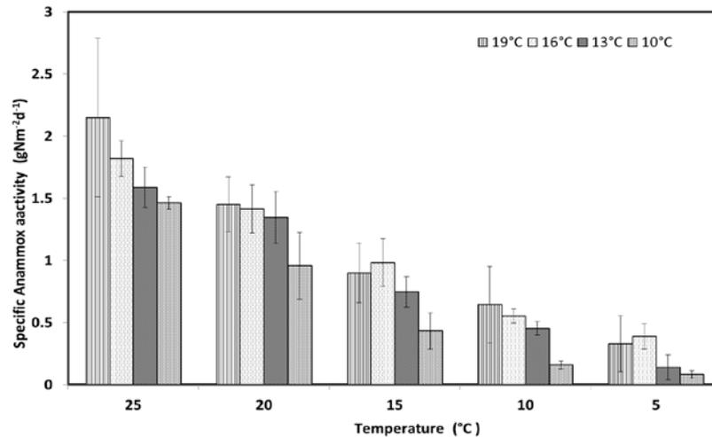
*Fig. 8: Effect of temperature on anammox activity (adapted from paper I).*
