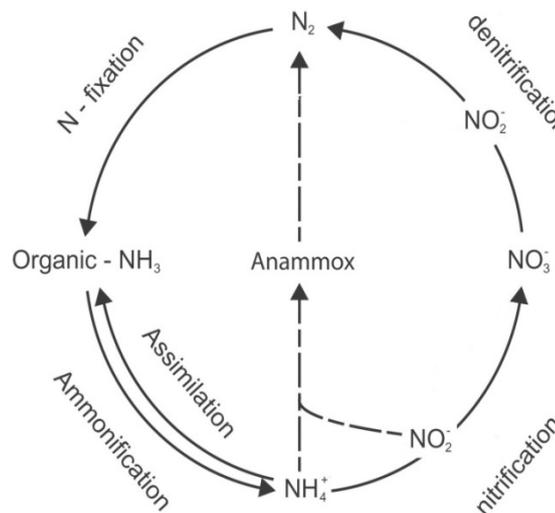
Fig. 1: Simplified Nitrogen cycle coupled with anammox (modification after Trimmer et al., 2003).
