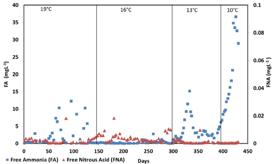
**Fig. 6: FA and FNA concentrations inside the MBBR operated at different temperature condition.**
