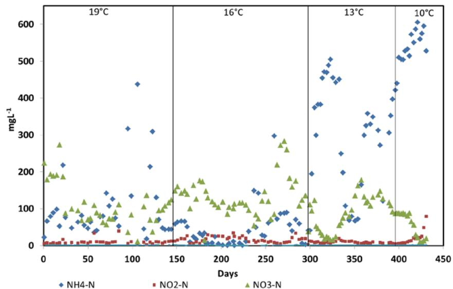
*Fig. 5: NH<sub>4</sub>-N, NO<sub>3</sub>-N and NO<sub>2</sub>-N concentration in the effluent at different operating temperatures in the MBBR.*
