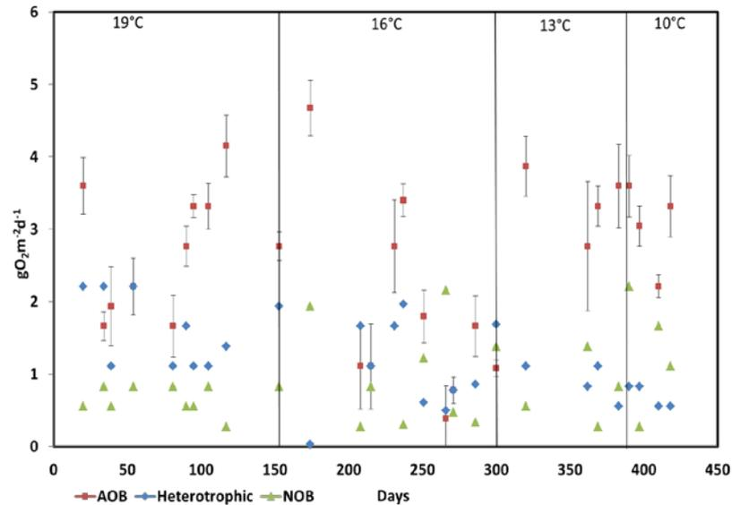
**Fig. 7: Activities of different groups of microorganism measured as OUR on the biocarriers during the pilot plant operation at different temperatures.**
