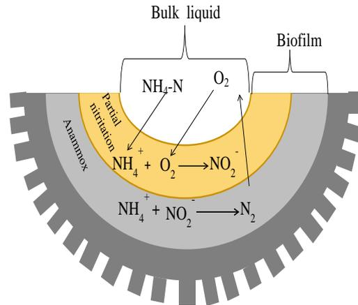
**Fig. 2: Partial nitrification/anammox process in biofilm system.**
