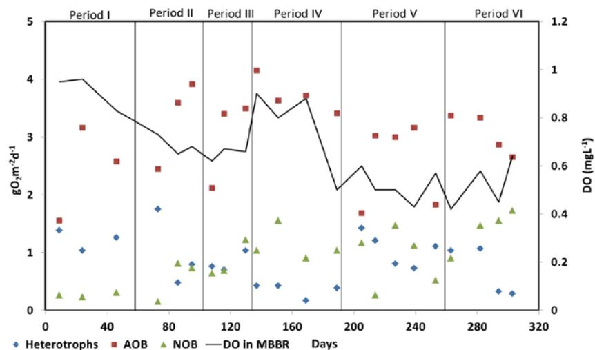
**Fig. 10: Activity of different groups of microorganism as measured by OUR on the biocarriers and DO concentration in the reactor in different periods.**
