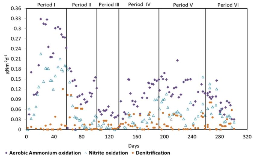
**Fig. 9: Measurement of aerobic ammonium oxidation, nitrite oxidation and denitrification in different periods.**
