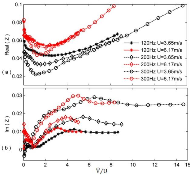
**Figure 6.** Measured normalized impedance in the orifice as a function of ratio between an acoustic particle velocity and mean flow velocity.
