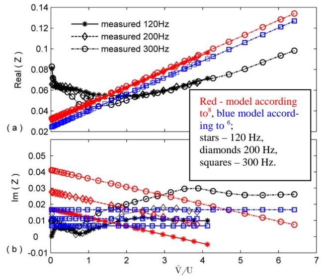
**Figure 7.** Normalized impedance in the orifice as a function of ratio between an acoustic particle velocity and mean flow velocity ( $U=6.17$  m/s).
