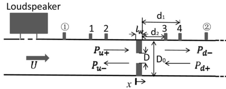
Figure 1. Test rig for measurement of orifice impedance.
