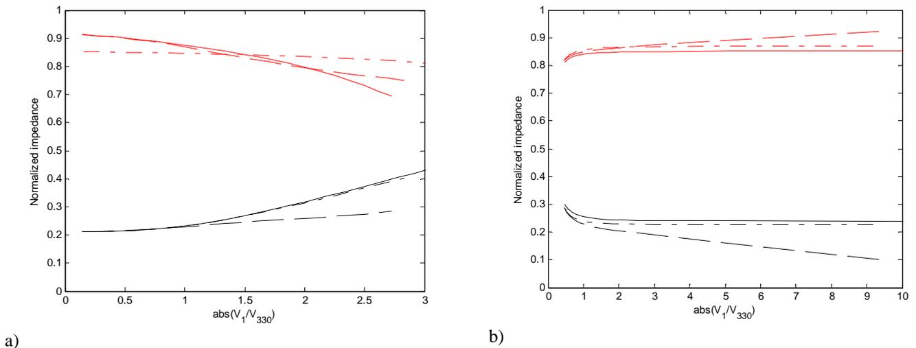
**Figure 4.** Normalized impedance for perforate with 2 % porosity at 330 Hz plotted against velocity ratio: Black – real part, red – imaginary part, solid line –  $V_I = V_{100}$ , dashed line –  $V_I = V_{110}$ , dashed-dotted line -  $V_I = V_{120}$ . a) Excitation at 330 Hz varied and excitation at the other frequencies kept constant, b) excitation at 100 Hz, 110 Hz and 120 Hz varied and excitation at 330 Hz kept constant.
