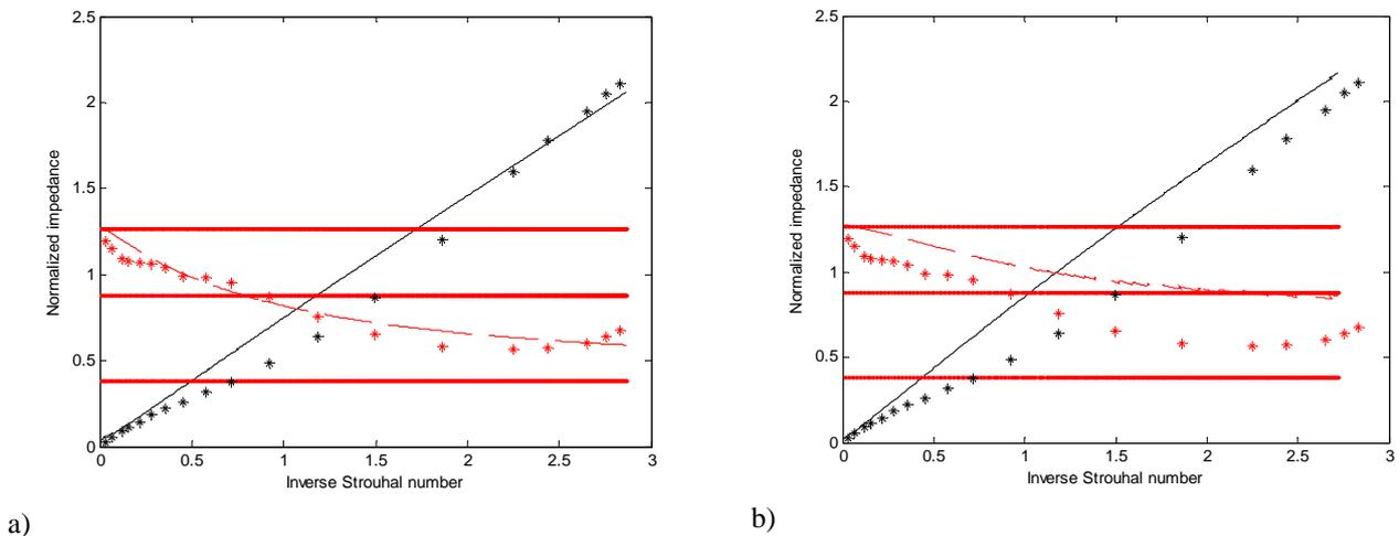
Figure 2. Normalized impedance for single orifice with 2.25 % porosity, plotted against inverse Strouhal number: black stars – measured real part, red stars – measured imaginary part, black solid line – simulated real part, red dashed line – simulated imaginary part, red thick lines – imaginary parts obtained assuming:  $l = l_0$ ,  $l = l_0 + l_w$  and  $l = 2l_0 + l_w$ . a) Jet length according to Eq. (4), b) jet length according to Eq. (3).
