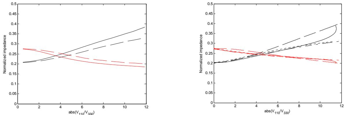
**Figure 5.** Real and imaginary parts of normalised impedance at 110 Hz for a perforate sample with 2% porosity plotted against velocity ratio for excitation at 110 Hz varied and excitation at 330 Hz kept constant: black – real part, red – imaginary part, solid line – phase at 330 Hz not shifted, dashed – phase at 330 Hz shifted 180 degrees, dashed-dotted – phase at 330 Hz shifted 60 degrees, dotted – phase at 330 Hz shifted 90 degrees. a) Measured, b) simulation.
