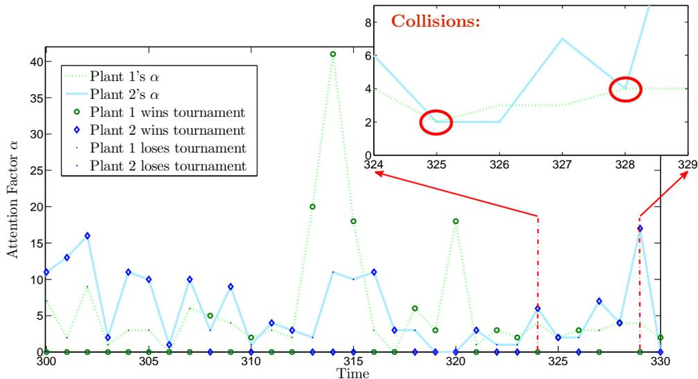
Fig. 10. A trace of the Attention Factors  $\alpha_k^j$  and the corresponding wins and losses in the tournaments, for both control systems in our hardware-in-the-loop experiment. The Attention Factors are obtained by quantizing a distortion-like function of the innovations (12). Note that two collisions are imminent from this trace.
