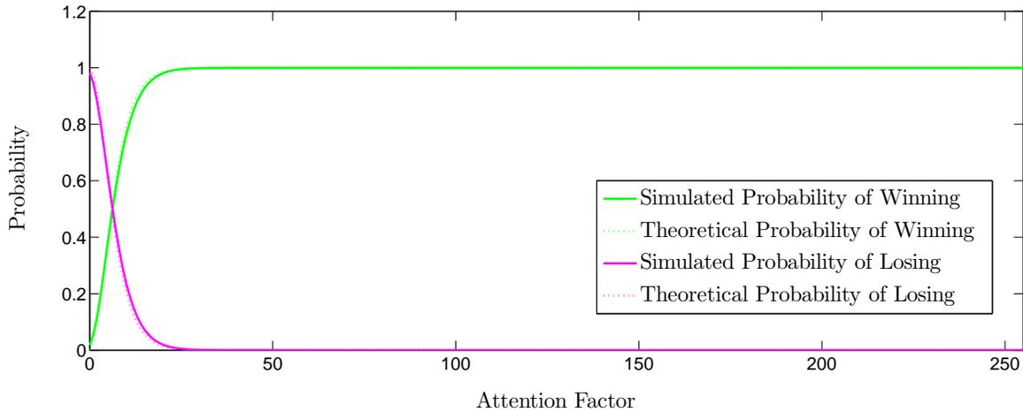
Fig. 6. The conditional probabilities of winning and losing in the tournament access mechanism are plotted above. Note that the simulated probabilities of these complimentary events match the analytical values. The probability of winning is a non-decreasing function of the Attention Factor, as shown in Lemma 3.4.
