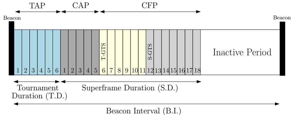
Fig. 5. Example of a superframe structure of the tournament-based IEEE 802.15.4 MAC. The tournament occurs during the TAP, while the transmission of the winner nodes is assigned to the T-GTSs, during the CFP. Scheduled communication for other network nodes is performed during the S-GTS, while best-effort transmissions occur during the CAP.
