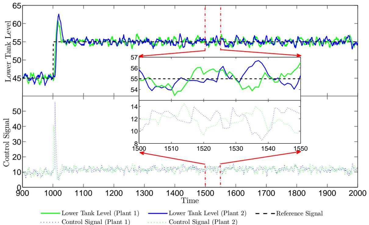
Fig. 9. A trace of the lower tank levels and controls, for both control systems, as obtained from the hardware-in-the-loop experiment. Notice that the control signal does not always correspond to the state, due to intermittent transmissions. Also, the reference tracking is successful for both stochastic systems, despite the two systems sharing a single slot for transmission.
