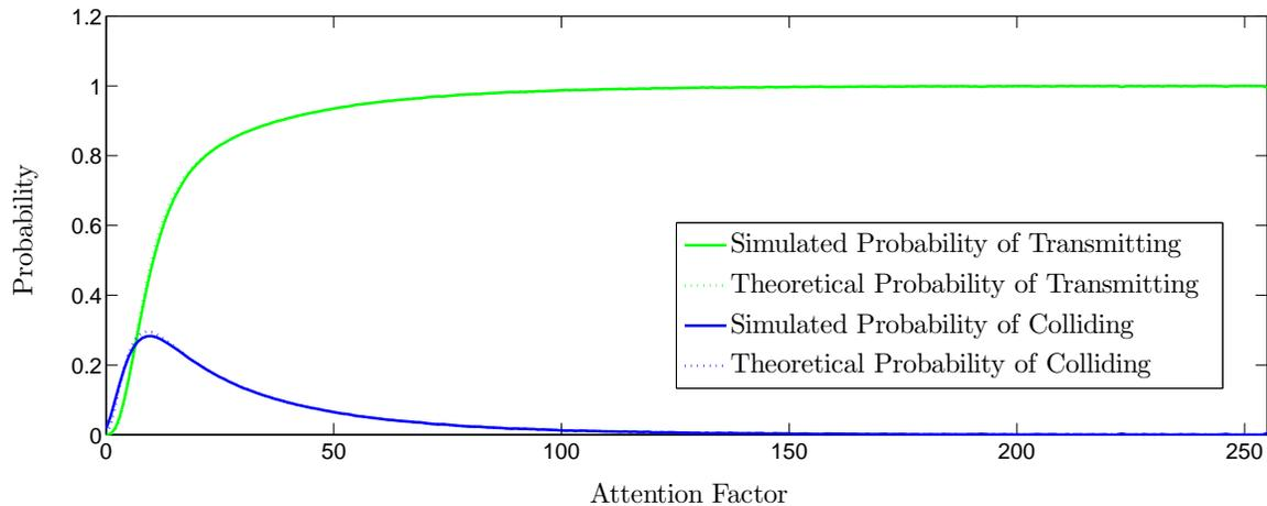
Fig. 7. The conditional probabilities of transmitting successfully and colliding in the tournament access mechanism are plotted above. Note that the simulated probabilities match the analytical values. The probability of transmitting is a non-decreasing function of the Attention Factor, as shown in Lemma 3.5.
