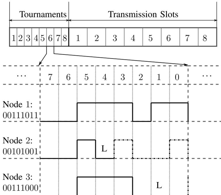
Fig. 3. The Frame Structure of the tournament access mechanism, with a tournament comprising of 8 priority bits, for each of the  $N_T = 8$  transmission slots. An example of a tournament is depicted here, with three nodes competing for the sixth transmission slot. Nodes 2 and 3 lose the tournament to node 1, and the symbol L depicts the priority bit during which the tournament is lost. Node 1 gets to transmit its data packet in the sixth transmission slot.
