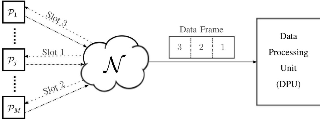
Fig. 1. An overview of a multiple access network ( $\mathcal{N}$ ) of plants ( $\mathcal{P}_j$ ),  $j \in \{1, \dots, M\}$ , with prioritized access in the MAC. The plant sensors communicate a priority to the network, which evaluates it distributedly, and suitably orders data packets in the frame.
