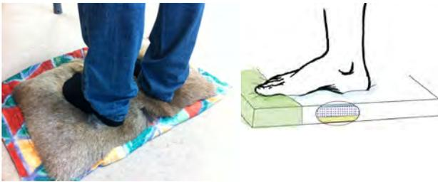
**Figure 4: Testing the prototype and an illustration of the different layers**
