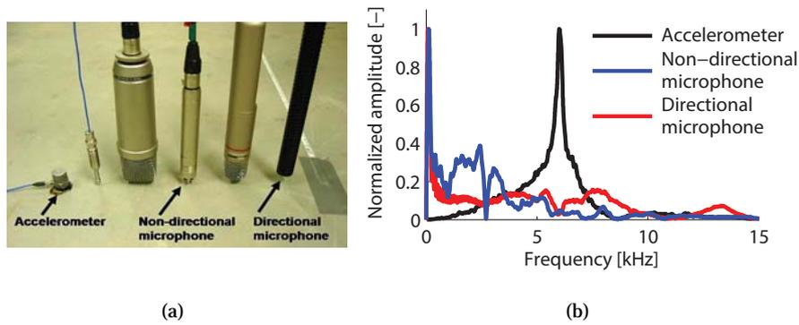
**Figure 3. (a) Three different used receivers marked with black arrows and (b) their corresponding frequency spectrum.**
