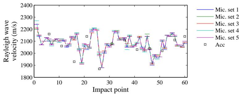
**Figure 10. Evaluated Rayleigh wave velocity along the survey line. The measurements are repeated five times to ensure high repeatability. The microphone array length at each position is illustrated with horizontal markers.**
