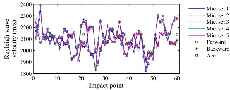
**Figure 11. Evaluated Rayleigh wave velocity from measurements performed in the forward and the backward direction. Accelerometer measurements are plotted for comparison.**
