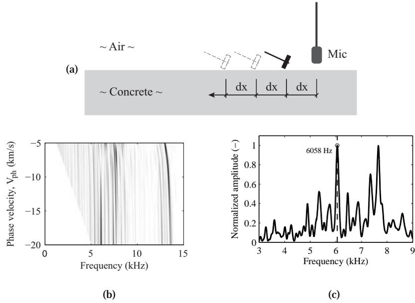
**Figure 15. (a) Schematic setup for the microphone case. (b) The amplitudes from the calculated dispersion curves for negative phase velocities were summed for each frequency and at last normalized and plotted in (c).**
