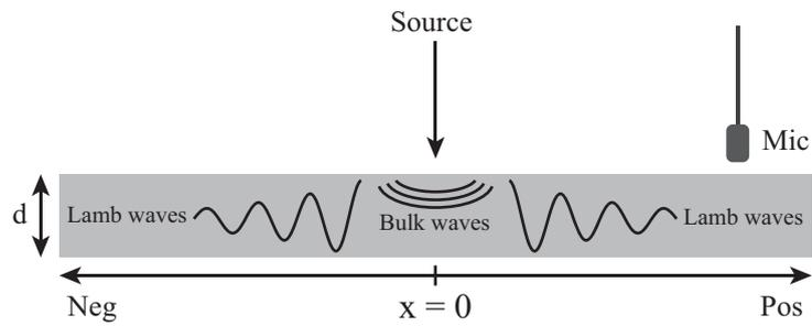
**Figure 6. A schematic picture of the measurement setup. A positive and negative direction is defined.**
