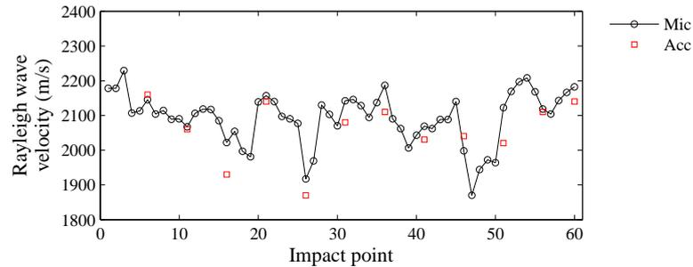
**Figure 12. Evaluated Rayleigh wave velocity averaged from forward and backward rolling measurements plotted in black. Accelerometer results are shown in red for comparison.**
