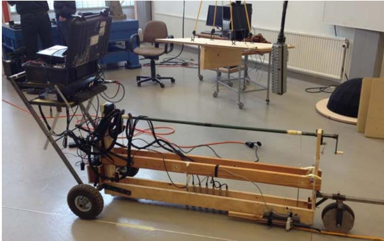
**Figure 8. Prototype trolley built by Ryden *et al.* (2008). The trolley enable air-coupled measurements performed while rolling.**
