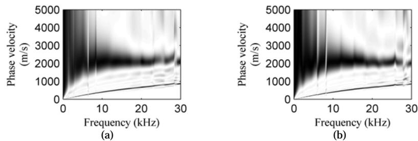
**Figure 9. Experimental dispersion curves from (a) accelerometer and (b) air-coupled microphones calculated using the MASW method.**
