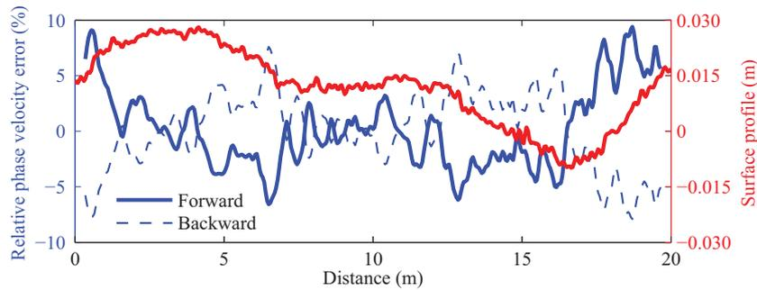
**Figure 13 : Relative phase velocity error (without unit) in calculated Rayleigh wave velocity for a synthetic periodic wave with a fix frequency of 12 kHz and a reference velocity of 2200 m/s.**
