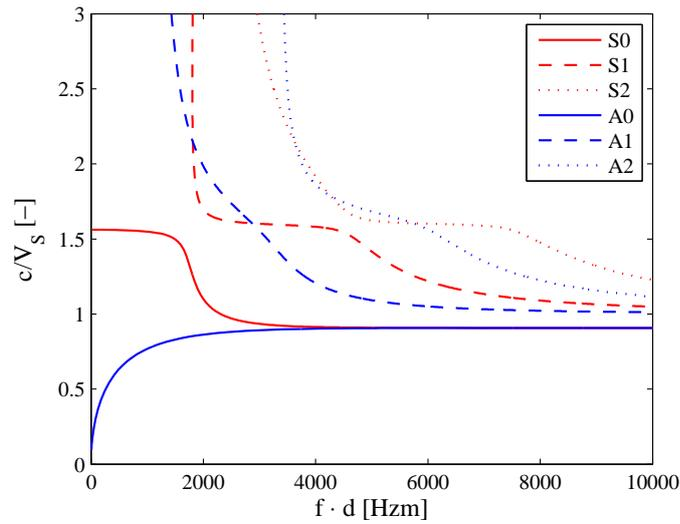
**Figure 5. Normalized dispersion curves for a plate with Poisson's ratio  $\nu = 0.18$ . The dispersion curves are valid for any plate thickness and shear wave velocity.**
