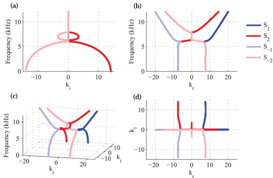
**Figure 7. Complex dispersion curves for a simulated plate with material parameters  $V_S = 2360$  m/s,  $d = 0.3$  m and  $\nu = 0.18$ . The curves are plotted in 3-D in (c) and their projections on the plane  $k_r = 0$  in (a),  $k_i = 0$  in (b) and finally  $f = 0$  in (d).**
