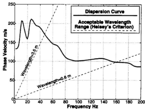
**Figure 2. Calculated dispersion curves using the SASW method. Only certain wavelengths from each measurement according to wavelength filter criteria can be used. (Results originally presented by Ganji *et al.* (1998))**
