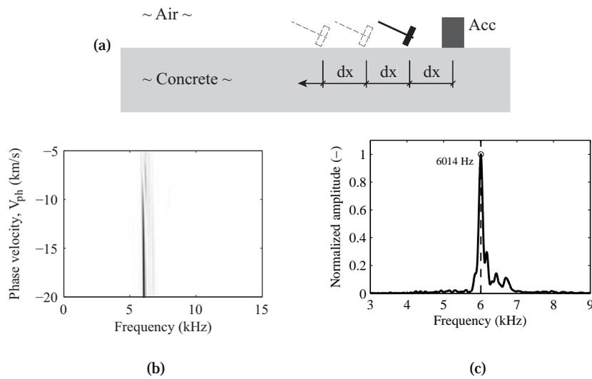
**Figure 14. (a) Schematic setup using accelerometer. (b) The amplitudes from the calculated dispersion curves for negative phase velocities were summed for each frequency and at last normalized and plotted in (c).**
