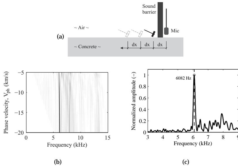
**Figure 16. (a) Schematic setup for the case using a microphone with a small sound barrier in front. (b) The amplitudes from the calculated dispersion curves for negative velocities were summed for each frequency and at last normalized and plotted in (c).**
