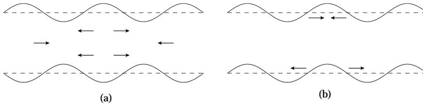
**Figure 4. Particle displacement of (a) symmetric and (b) asymmetric Lamb wave modes.**
