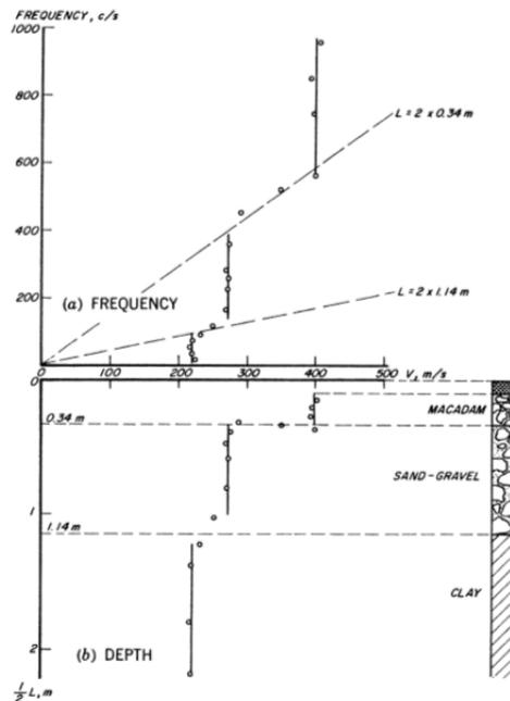
**Figure 1. Estimated dispersion curves using the steady state measurements. Original figure presented by Heukelom and Foster (1960).**
