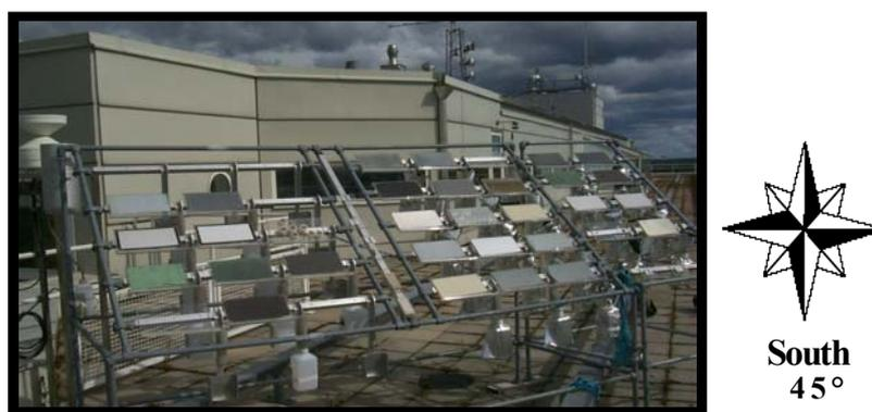
Figure 6. Test site for metal runoff studies (field exposure).
