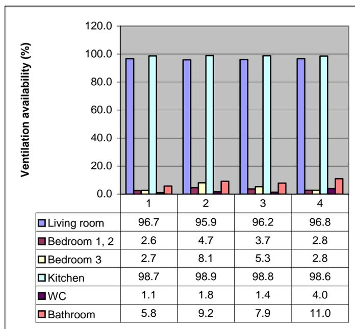
Figure 24. The ventilation availability in different rooms at different opening configurations. Living room door open. 1) basic opening area, 2) supply openings to bedrooms doubled, 3) overflow openings to bedrooms doubled and 4) overflow openings to WC/bathroom doubled.
