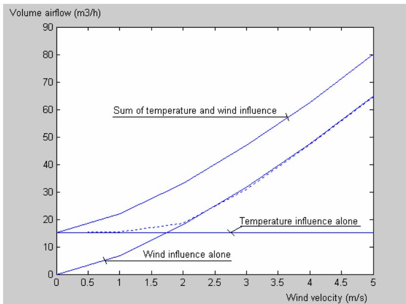
Figure 14. Combined air leakage flow (dotted lines).  $r = 1, s = 0$ .
