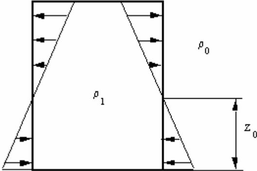
Figure 1. Buoyancy induced pressure profile across the building envelope.
