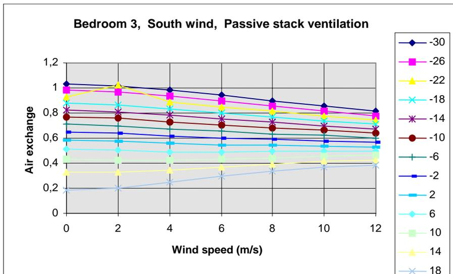
Figure 21. Air exchange in bedroom 3 at different outside temperatures. Natural ventilation and wind from south.
