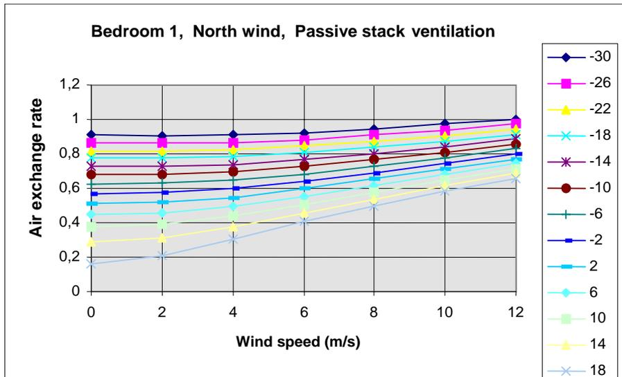
Figure 20. Air exchange in bedroom 1 at different outside temperatures. Natural ventilation and wind from north.
