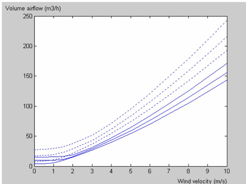
Figure 11. The air leakage with two values on the leakiness ratio  $s$ ,  $s = 0$  (continuous lines) and  $s = 0.6$  (dotted lines), and three temperature differences,  $\Delta T = 10, 30$  and  $50$  K. Higher  $\Delta T$  means higher airflow. Combined temperature and wind influence.  $n = 0.7, r = 1$ .
