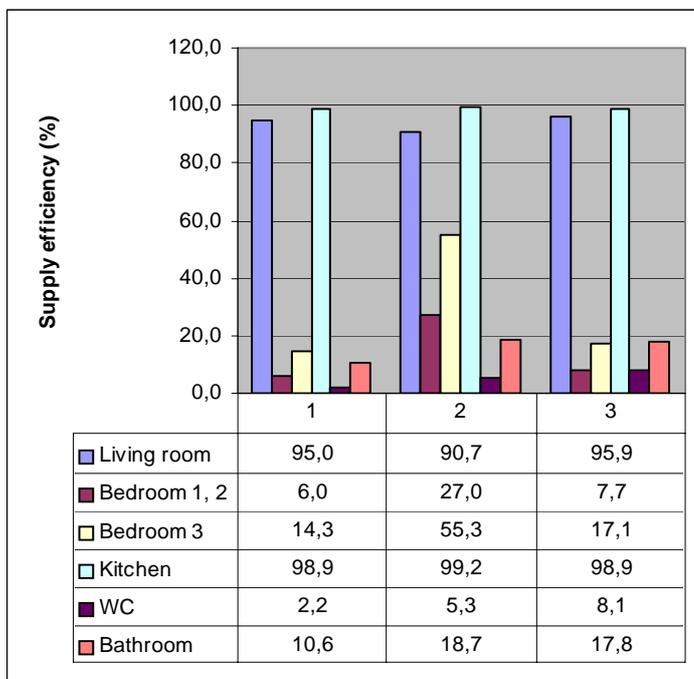
Figure 26. The ventilation availability in different rooms at different opening configurations. Living room and bedroom doors open. 1) basic opening area, 2) supply openings to bedrooms doubled and 3) overflow openings to WC/bathroom doubled.
