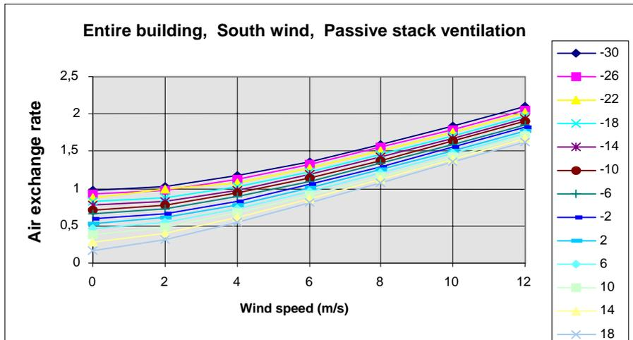
Figure 18. Air exchange rate in the entire building at different outside temperatures. Natural ventilation and wind from south.
