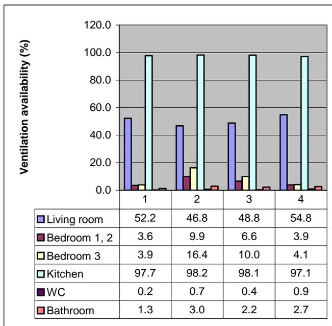
Figure 23. The ventilation availability in different rooms at different opening configurations. Living room door closed. 1) basic opening area, 2) supply openings to bedrooms doubled, 3) overflow openings to bedrooms doubled and 4) overflow openings to WC/bathroom doubled.
