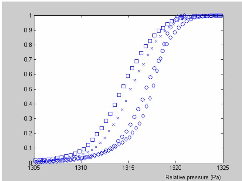
Figure 29. Pressure distribution in WC with extended chimney height compared to mechanical exhaust from WC/bathroom.  $\diamond$  = mechanical exhaust,  $o$  = 0 m,  $x$  = 3 m and  $\square$  = 5 m extra chimney height. Pressure relative to 100 000 Pa.
