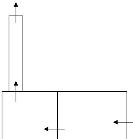
Figure 3. Simplified airflow through a building.
