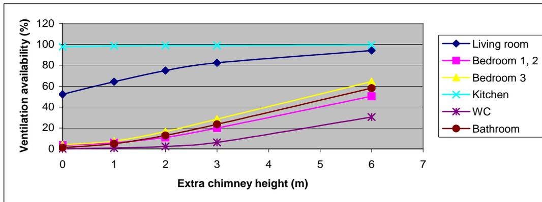
Figure 22. Influence on the ventilation availability from increasing chimney height.
