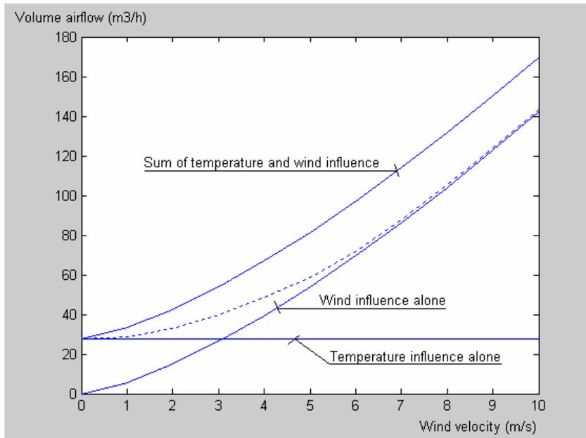
Figure 13. Combined air leakage flow (dotted line).  $r = 3, s = 0.6$ .
