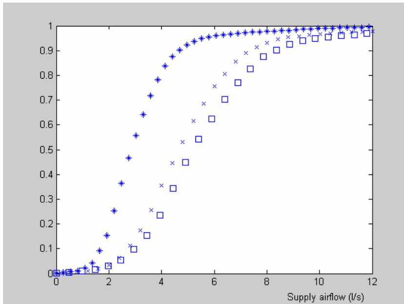
Figure 28. Cumulative distribution of air supply to bedroom 1 and 2. Basic configuration with living room door open (\*), with 140 mm<sup>2</sup> supply openings in bedrooms (x) and with 140 cm<sup>2</sup> supply and overflow openings (◻).
