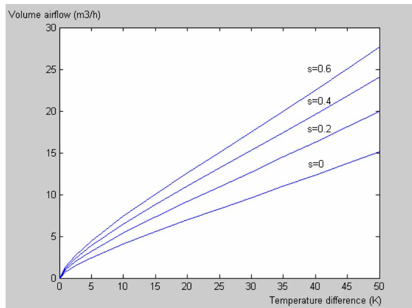
Figure 8. The air leakage with different values on the leakiness ratio  $s$ . Temperature influence alone.  $n = 0.7$ .
