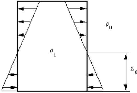
Figure 6. The temperature dependent pressure distribution across the building shell.
