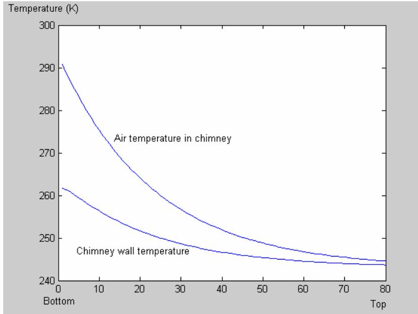
Figure 5. Temperatures in air and chimney wall. Outside temperature is  $-30\text{ }^{\circ}\text{C}$ . 5 mm chimney without insulation.
