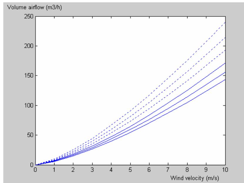
Figure 9. The air leakage with two values on the leakiness ratio  $s$ ,  $s = 0$  (continuous lines) and  $s = 0.6$  (dotted lines), and three temperature differences,  $\Delta T = 10, 30$  and  $50$  K. Higher  $\Delta T$  means higher airflow. Wind influence alone.  $n = 0.7, r = 1$ .
