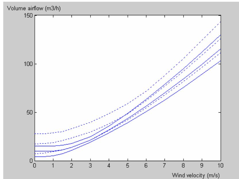
Figure 12. The air leakage with two values on the leakiness ratio  $s$ ,  $s = 0$  (continuous lines) and  $s = 0.6$  (dotted lines), and three temperature differences,  $\Delta T = 10, 30$  and  $50$  K. Higher  $\Delta T$  means higher airflow. Combined temperature and wind influence.  $n = 0.7, r = 3$ .
