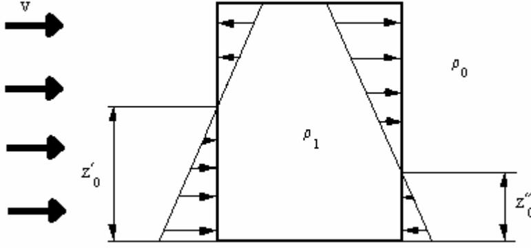
Figure 7. The pressure distribution across a building with combined temperature and wind influence.
