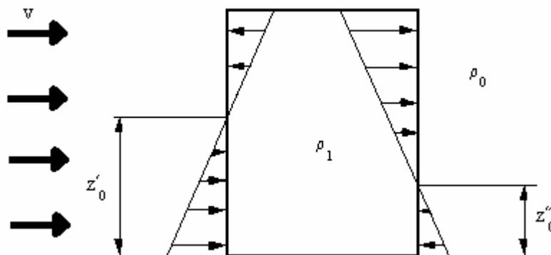
Figure 2. Pressure distribution and neutral levels at combined temperature and wind influence.
