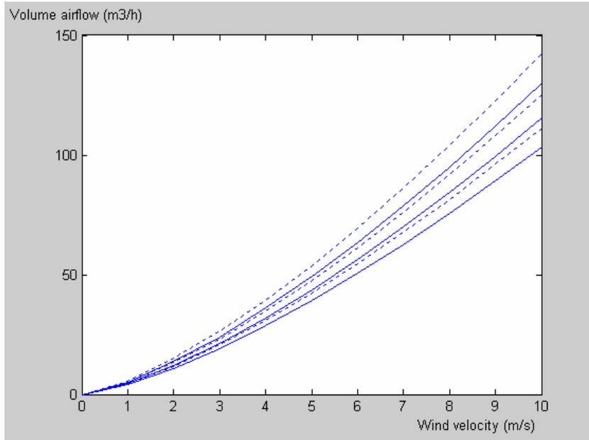
Figure 10. The air leakage with two values on the leakiness ratio  $s$ ,  $s = 0$  (continuous lines) and  $s = 0.6$  (dotted lines), and three temperature differences,  $\Delta T = 10, 30$  and  $50$  K. Higher  $\Delta T$  means higher airflow. Wind influence alone.  $n = 0.7, r = 3$ .
