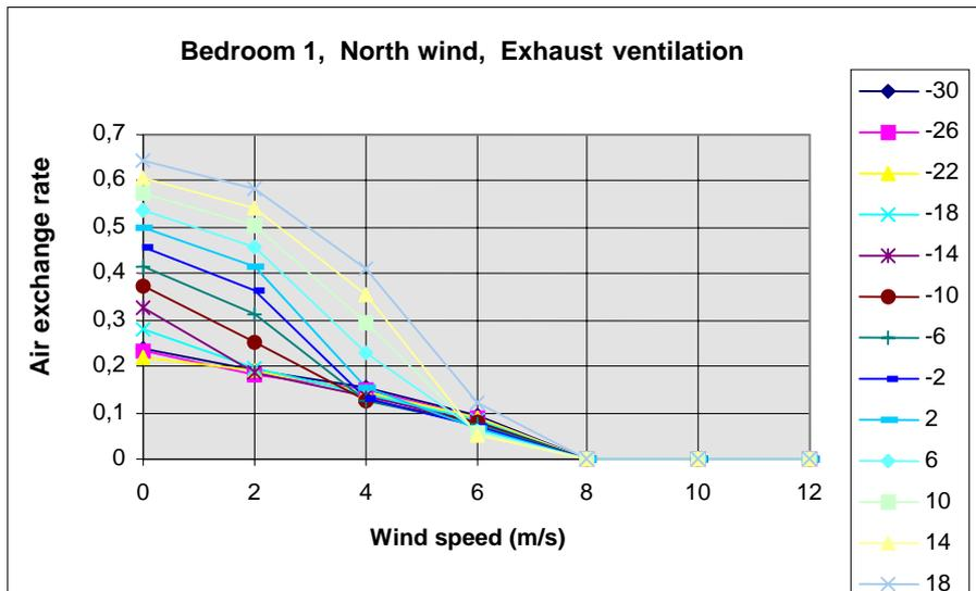
Figure 19. Air exchange in bedroom 1 at different outside temperatures. Exhaust ventilation and wind from north.
