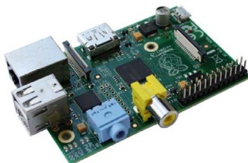
**Figure 1.** The Raspberry PI Model B (source: Raspberry PI website).
