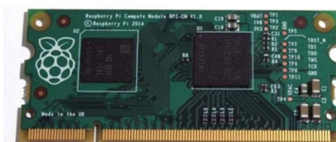
**Figure 7.** The RPI Compute Model;  $67.6 \times 30$  mm board as DDR2 SODIMM (Source: Raspberry PI website).
