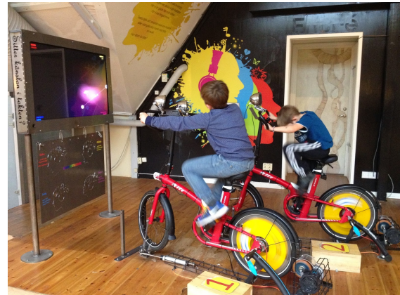
Figure 1. The Musikcyklarna installation with two users at the Experiment. Notice the two loudspeakers on the handlebars, the rotation sensor for the front wheel and the magnetic field sensor behind the rear wheel. The display shows two blobs corresponding to the position of each bicycle in the activity-valence space
