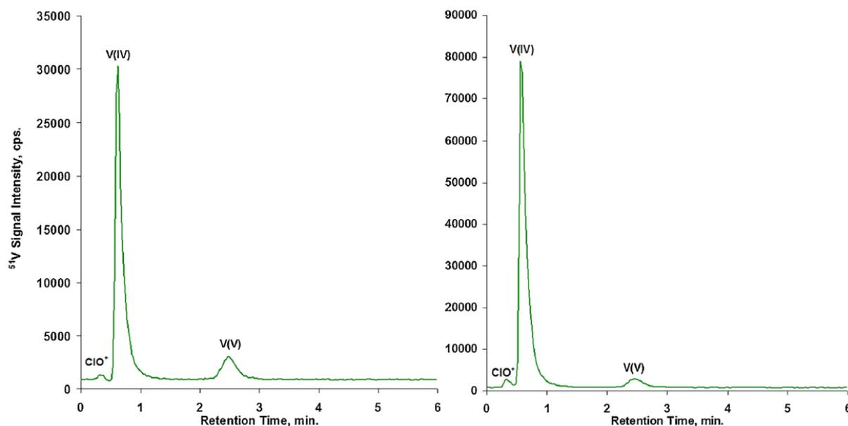
**Figure 2.** HPLC-ICP-MS chromatograms of water extracts of the two blast furnace slags, M-Kalk (left) and Merit 5000 (right). The  $^{35}\text{Cl}^{16}\text{O}^+$  interference is resolved chromatographically and does not affect the detection of the two species of interest, i.e., V(IV) and V(V).
