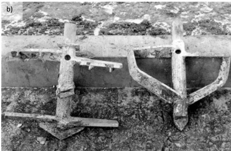
Figure 1: (a) Typical machinery for manufacturing lime-cement columns; (b) Pin drill and Swedish standard mixing tool (courtesy of Skanska AB; Larsson et al. 2005a).
