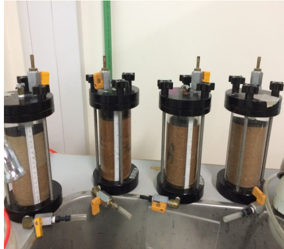
Fig.6. Samples used for the constant head permeability test, (AUD, 2014).
