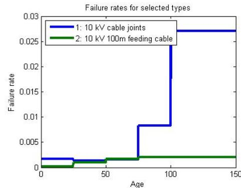
**Figure 4** The failure rates for 100 m cables and cable joints for the population in the case study. The failure rate is stated in failures per year and per cable joint or 100 m cable.
