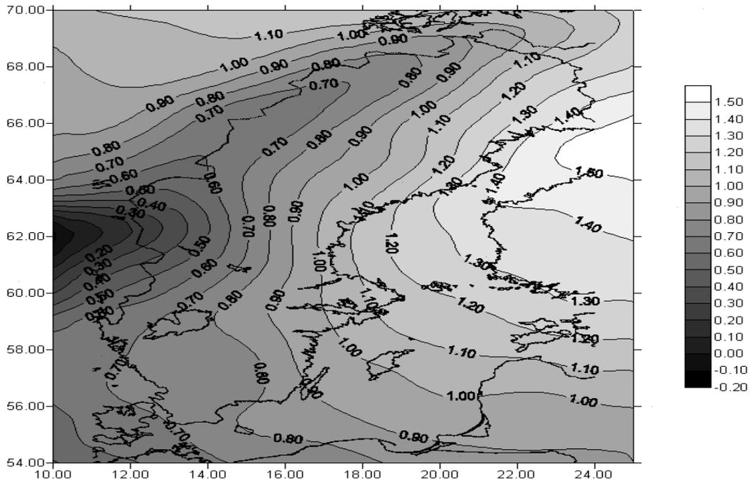
Figure 5.8: The total atmospheric effect on the geoid. Contour interval is 0.1 cm.
