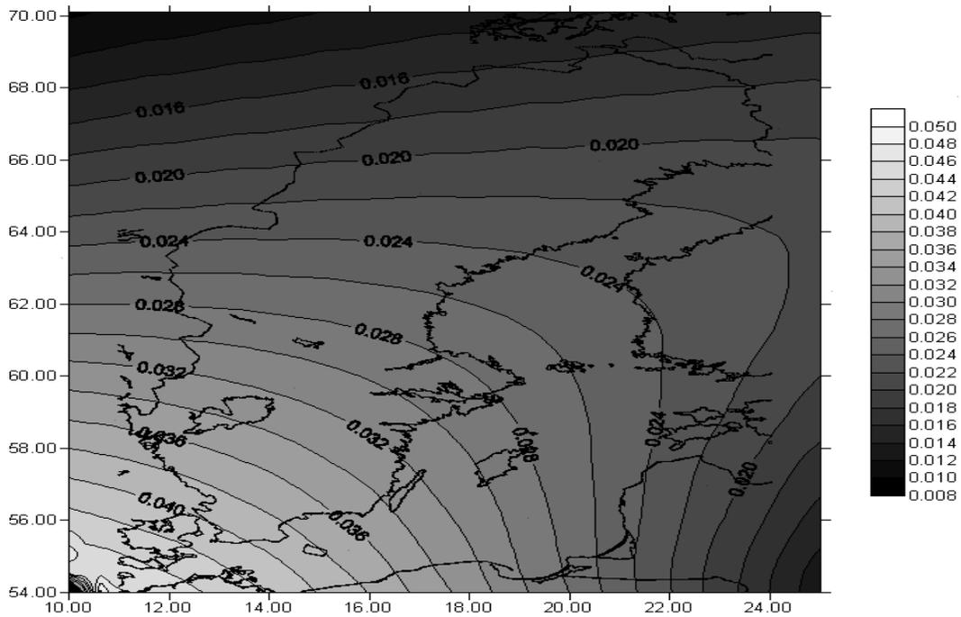
Figure 5.5: The ellipsoidal correction. Contour interval is 0.002 mGal.
