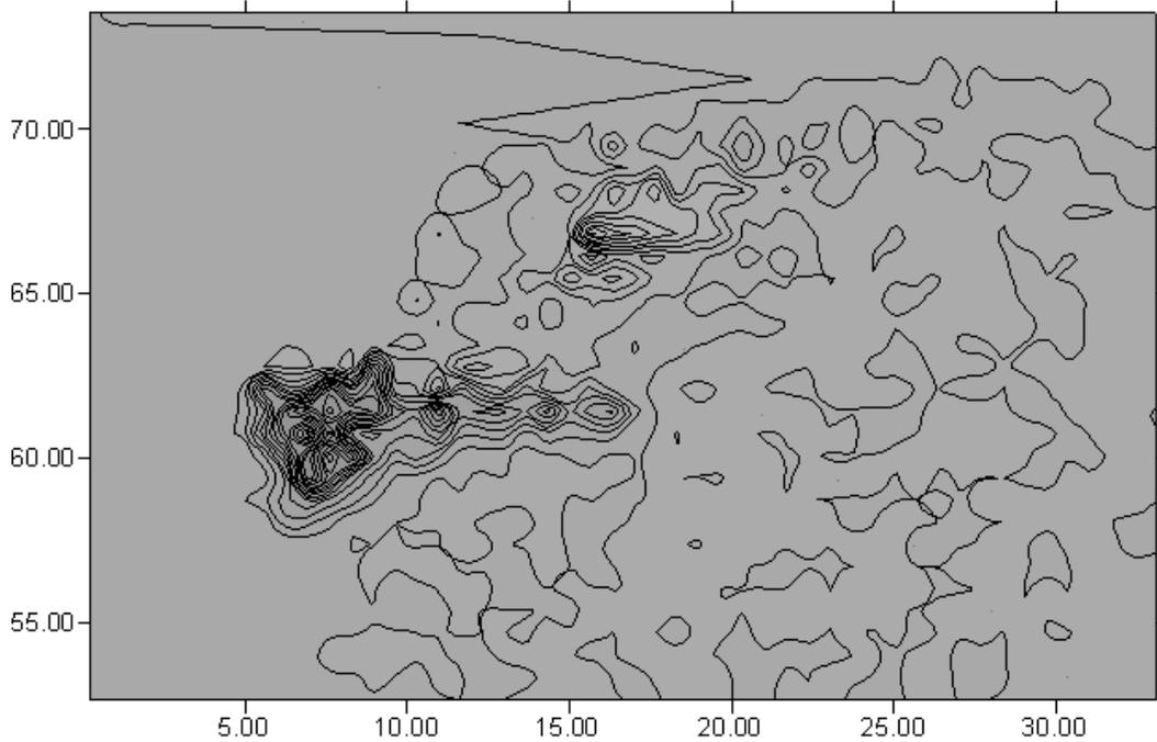
Figure 5.6: The difference between gravity anomalies on the Earth's surface and on the geoid. Contour interval is 6 mGal.
