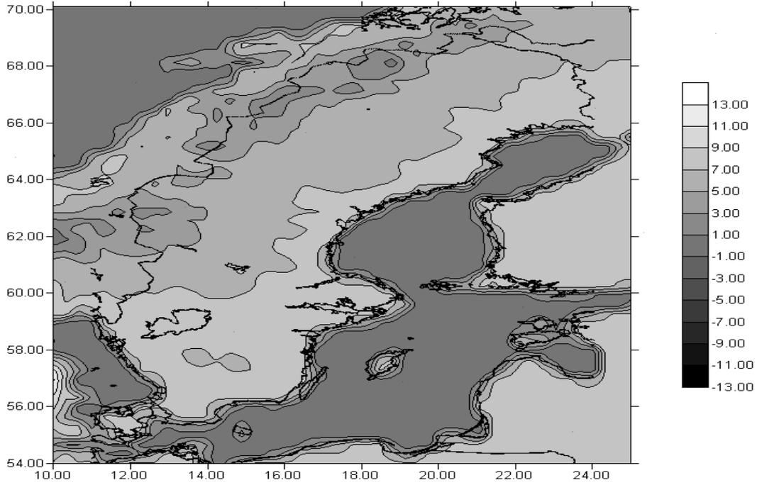
Figure 5.7: The primary indirect terrain effect. Contour interval is 2 cm.
