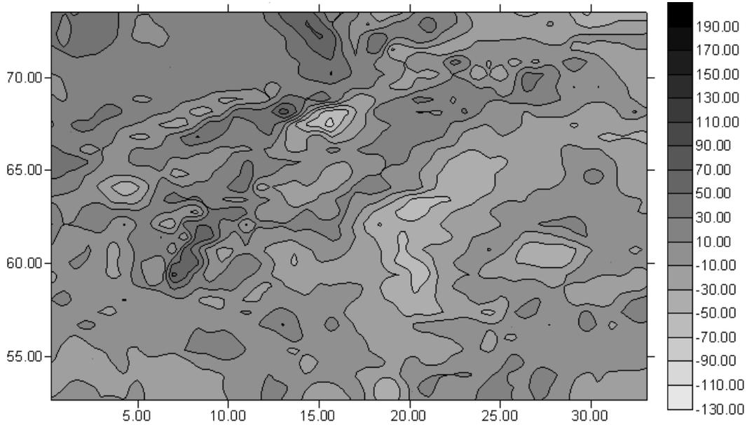
Figure 5.1: The mean free-air gravity anomalies over Scandinavia. Contour interval is 20 mGal.
