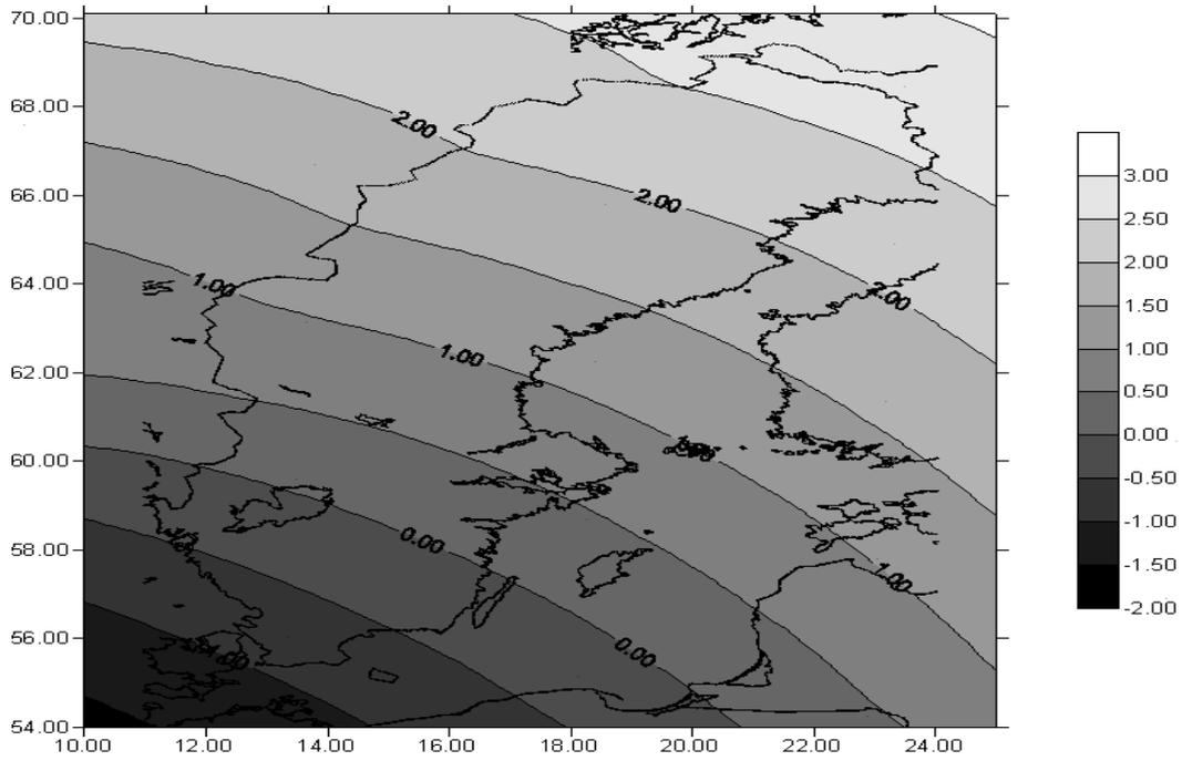
Figure 5.4: The secondary direct terrain effect on the geoid. Contour interval is 0.5 cm.
