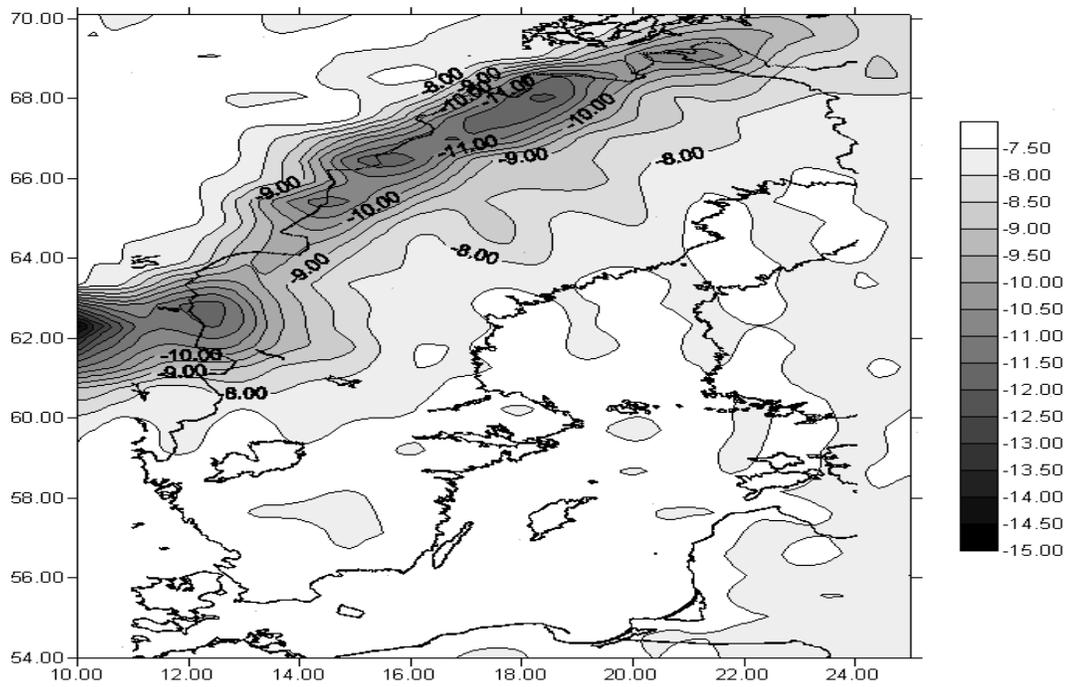
Figure 5.3: The direct terrain effect on geopotential. Contour interval is 0.5 cm.
