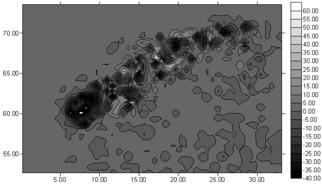
Figure 5.2: The direct terrain effect. Contour interval is 5 mGal.
