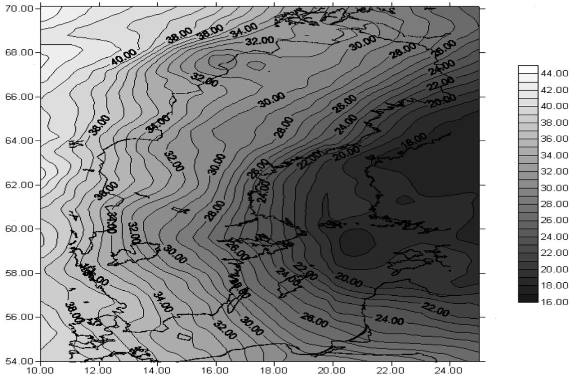
Figure 5.10: The final gravimetric geoid determined by the refined least squares estimator. Contour interval is 1 m.
