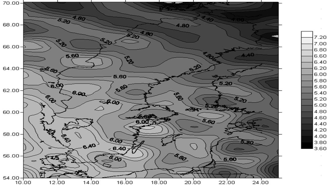
Figure 5.9: The correction due to the truncation of Stokes's integral to a spherical cap with radius  $\psi_0 = 6^\circ$ . Contour interval is 0.2 cm.
