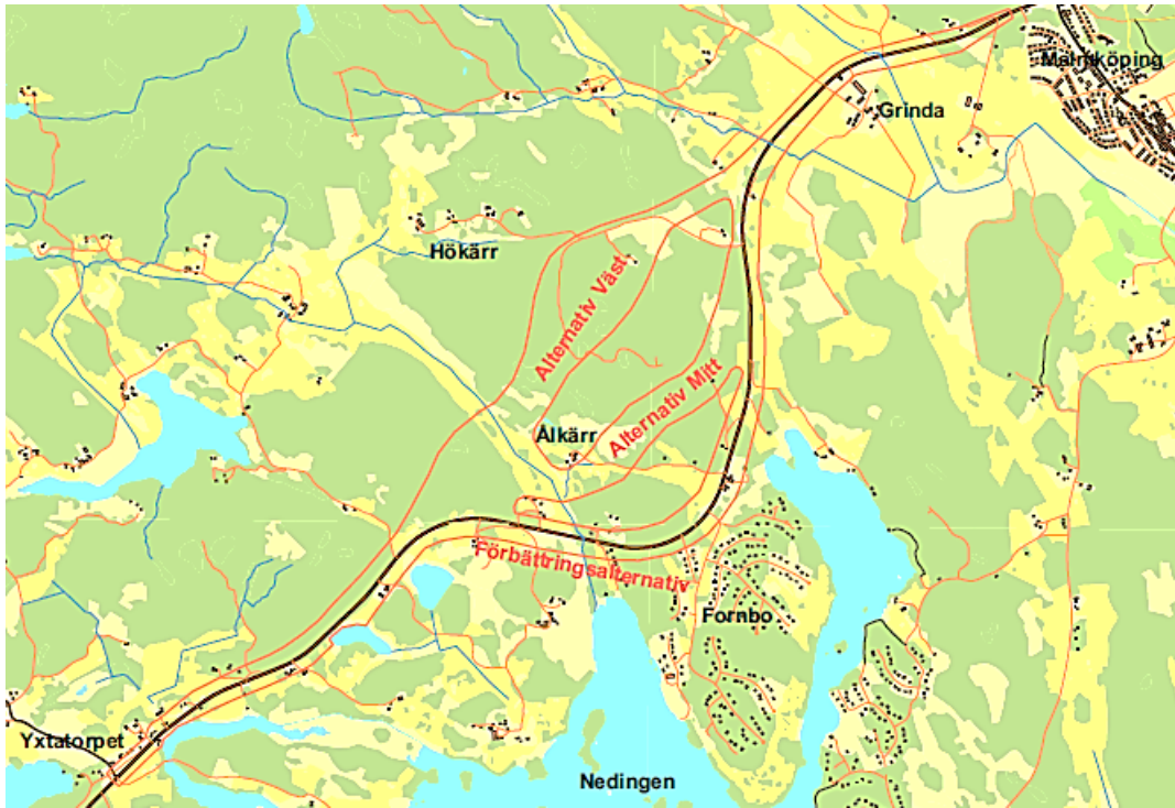
Figure 3: Schematic representation of road corridor alternatives for a section of Road 55 between Yxtatorpet and Malmköping
