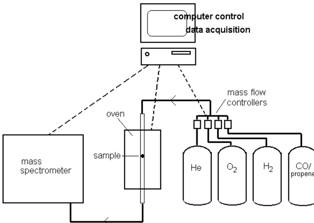
Fig. 17. A schematic drawing of catalytic reactor set-up.
