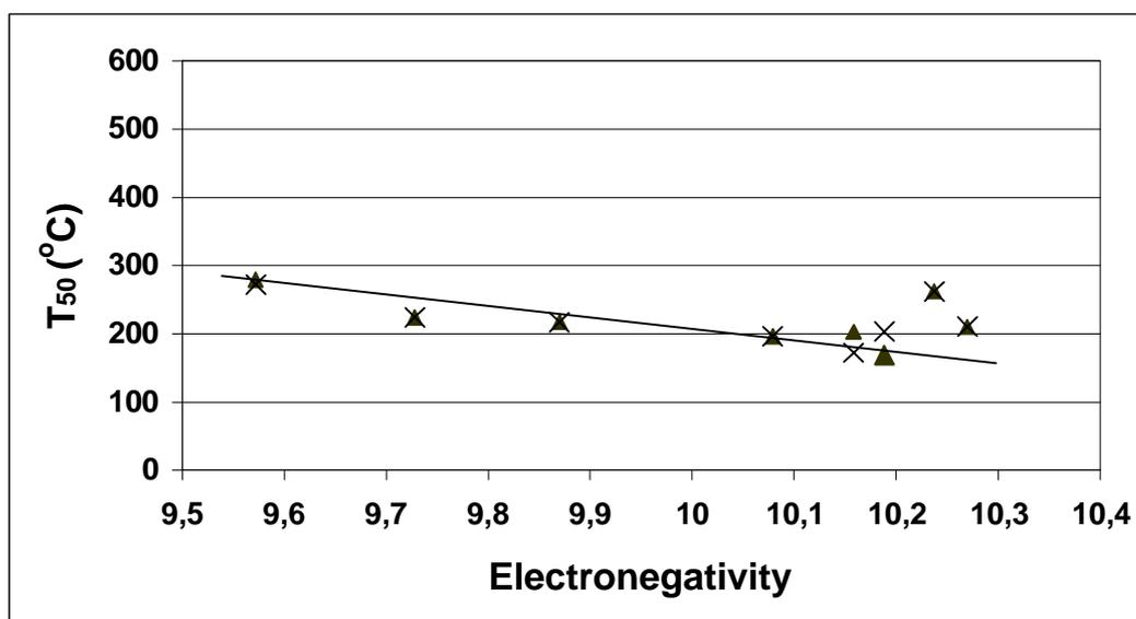
Fig. 28. Ignition temperature for carbon monoxide and propene combustion on palladium loaded doped ceria catalysts as a function of electronegativity.
