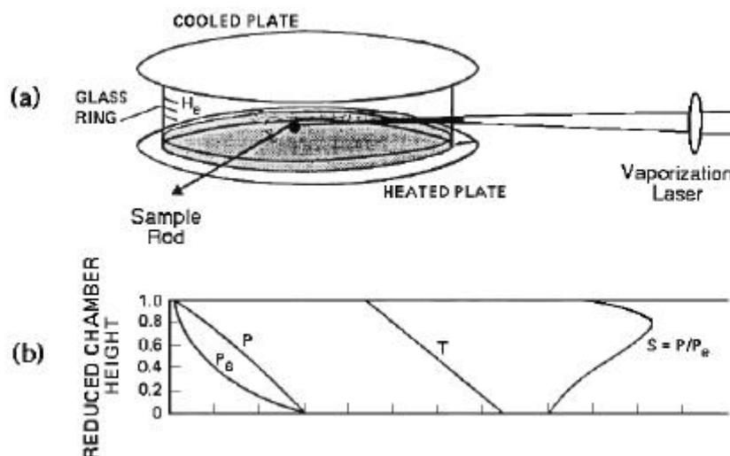
Fig. 15. (a) A diagram of the diffusion cloud chamber, (b) temperature and pressure profiles in the chamber.
