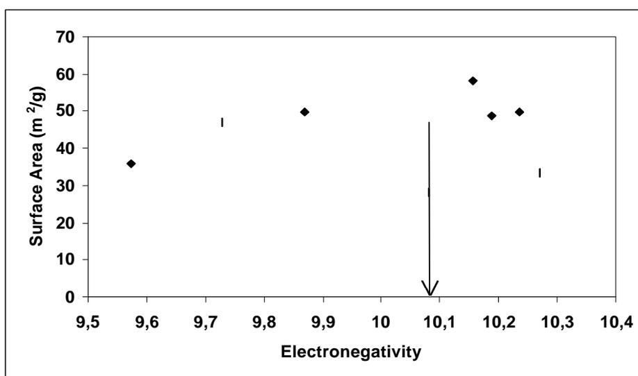
Fig. 26. a. Light-off temperature for carbon monoxide oxidation as a function of surface area, b. Surface area as a function of electronegativity (electronegativity of ceria is marked with an arrow).
