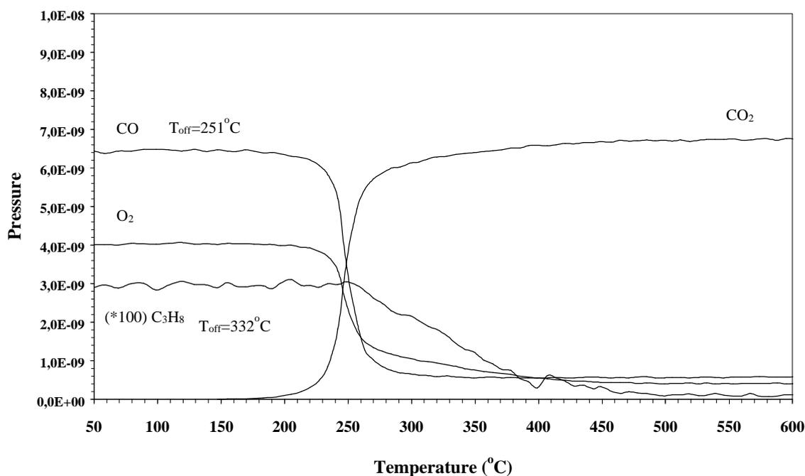
Fig. 29. Conversion of CO and  $\text{C}_3\text{H}_6$  on spinel catalysts, the light off temperature was  $251^\circ\text{C}$  for CO and  $332^\circ\text{C}$  for  $\text{C}_3\text{H}_6$  combustion.
