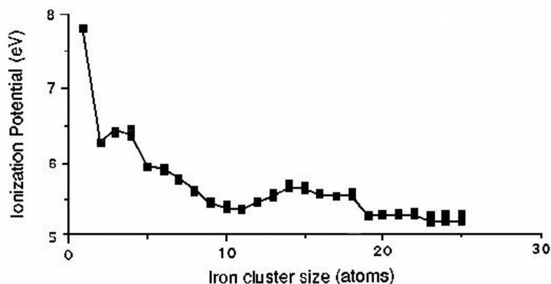
Fig. 3. The ionization potential of iron clusters as a function of cluster size. [6]
