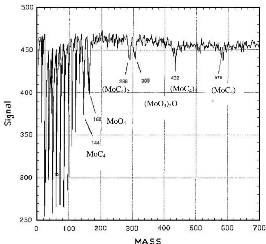
Fig. 20. Mass spectrum of sample prepared by laser evaporation of Mo in isobutylene atmosphere. The presence of MoC<sub>n</sub> as well as molybdenum oxides can be seen.
