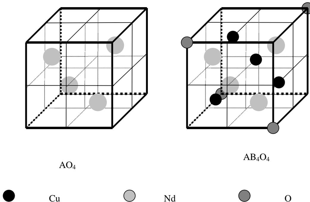
Fig. 11. Crystal structure of  $\text{Nd}_{1.5}\text{Ca}_{0.5}\text{CuO}_4$  spinel.
