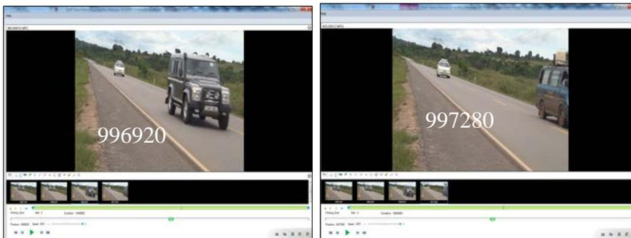
c) Passing vehicle reaches beginning of 24m mark    d) Passed vehicle reaches beginning of 24m mark
