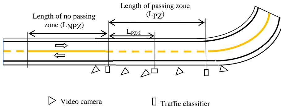
**Fig. 3-3: Field layout and equipment used for speed and passing data collection**
