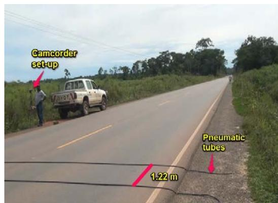
c) Traffic classifiers and pneumatic tubes placed across the highway pavement
