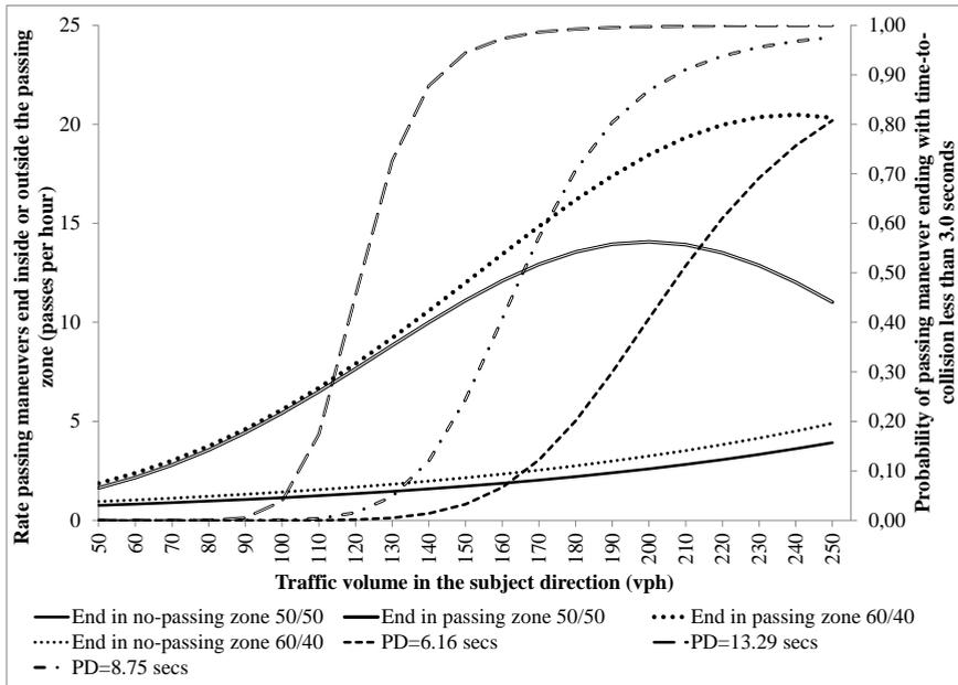
**Fig. 4-1: Rate of passing maneuvers that end inside or outside the passing zone and the probability of ending with time-to-collision less than 3.0 seconds as a function of traffic volume in the subject direction**
