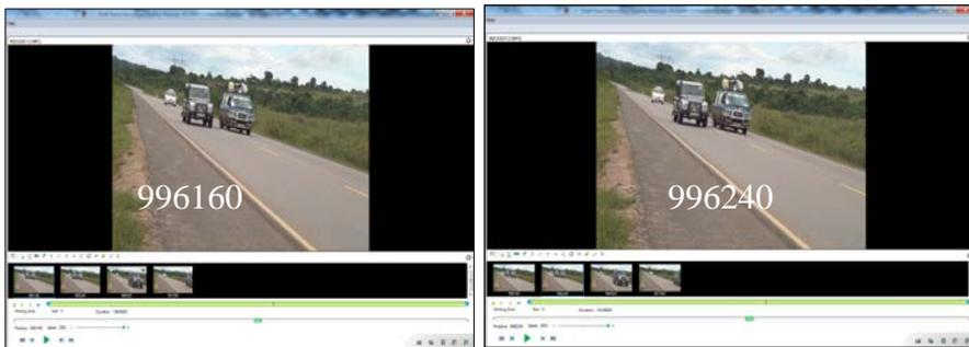
a) Passed vehicle reaches end of 24m mark    b) Passing vehicle reaches end of 24m mark
