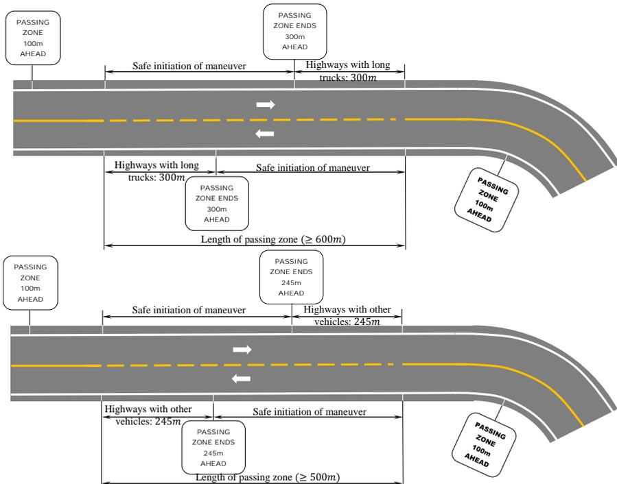
**Fig. 4-2: Recommended additional signage in the passing zone**
