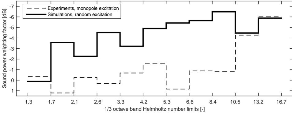
Figure 3.8: The 1/3 octave frequency band acoustic power weighting factors as a function of the 1/3 octave band limiting Helmholtz numbers. Solid line: Simulated weighting factors for multi-modal excitation based on 4096 microphone configurations, Paper IV [43]. Dashed line: Weighting factors for monopole excitation from experiments, Paper II [39].
