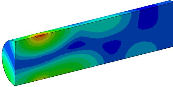
Figure 3.7: Sound pressure distribution at the frequency of 770 Hz. That corresponds to the Helmholtz frequency of 1.8. The colours in the figure describe magnitude of the sound pressure; ranging from higher sound pressure (red) to the lower sound pressure (blue). The excitation of the mode shape  $\psi_{10}$  ( $f_{10,cut-on} \approx 788$  Hz) can be noted from the sound pressure variation.
