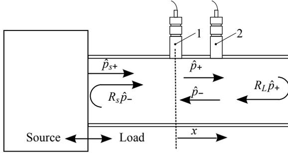
Figure 2.1: Schematic of the acoustic one-port source and the propagating waves. In the low frequency plane wave range, the downstream (+) and upstream (-) propagating waves can be separated using the two-microphone method.
