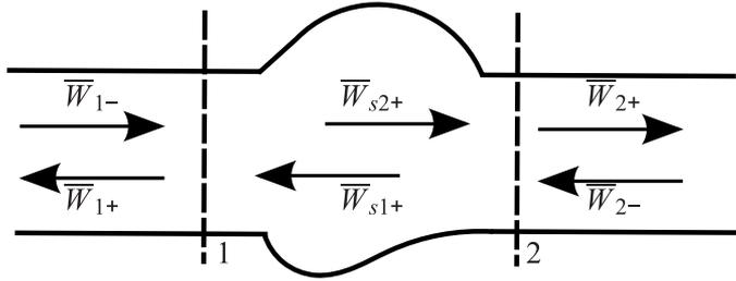
Figure 2.3: Directions of the sound power flow in an acoustic two-port. The power is positive when flowing out of the port.
