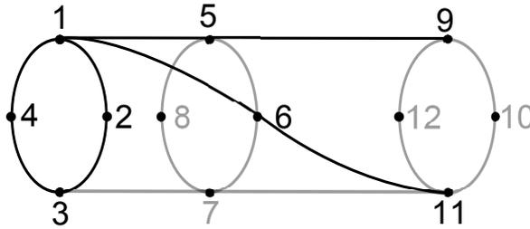
Figure 3.3: The microphone configurations used in the spectra averaging. 1-6-11 is the spiral microphone setup.
