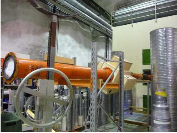
Figure 3.1: Test-rig (orange pipe) for the high frequency acoustic power weighting factor determination. The absorbing end is to the left and the right-hand opening is connected to a reverberation room.
