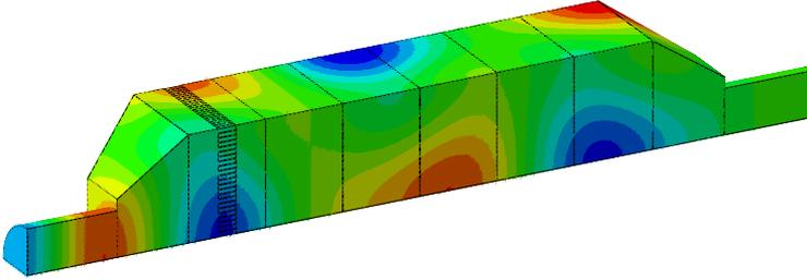
Figure 3.15: Acoustic pressure distribution of the tested ATD at the frequency of  $He = 1.50$  for 1 Pa excitation at the inlet (left end). The sound reflections in the ATD are strong, which can be seen as weak wave propagation at the outlet duct. From Paper V [40].
