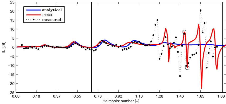
Figure 3.14: The analytical, FEM and measured insertion loss of the test ATD as a function of the Helmholtz number, from Paper V [40]. The cut-on frequency of the first non-plane wave mode in the chamber is denoted with the first thick vertical line. The second thick vertical line denotes the cut-on frequency of the first non-plane wave mode in the inlet duct.
