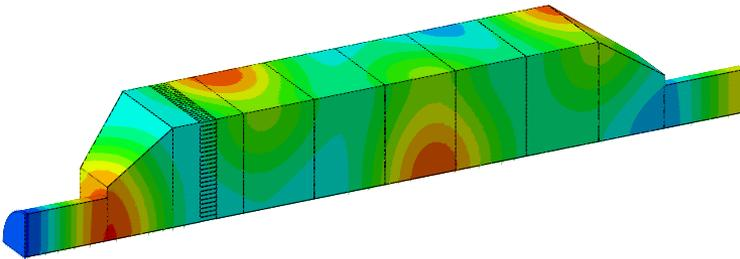
Figure 3.16: Acoustic pressure distribution of the tested ATD at the frequency of  $He = 1.53$  for 1 Pa excitation at the inlet (left end). The sound transmission through the ATD is strong, which can be seen as propagating waves at the outlet duct. From Paper V [40].
