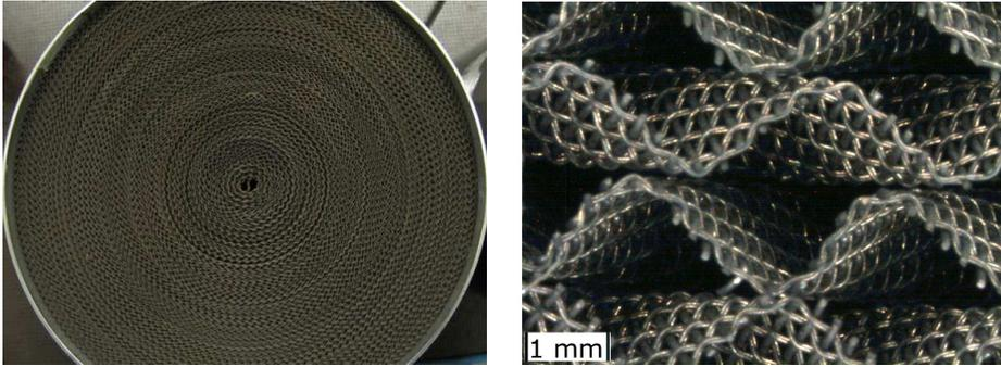
Figure 3.17: POC-X type filter (left) and microscope photograph of the substrate cells formed from the metallic wire mesh screens (right), see Paper VI [42].
