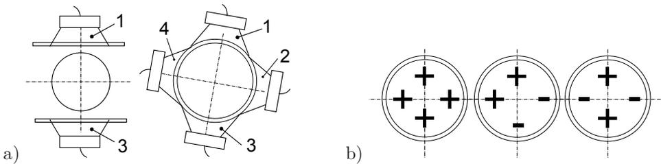
Figure 3.2: a) The loudspeaker setup for generating the monopole, dipole and quadrupole source types. b) Phasing of the four loudspeakers to generate acoustic source types, from left to right: monopole, dipole, and quadrupole.
