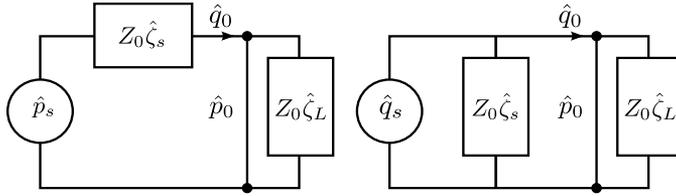
Figure 2.2: Electro-acoustic analogy for a linear time-invariant one port source model. Pressure source (left), volume velocity source (right).
