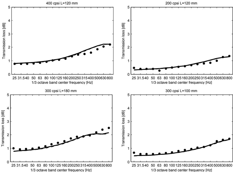
Figure 3.18: The simulated (lines) and measured (marks) transmission losses of the tested filters in the plane wave frequency range. The uncorrected simulation results (with the correction factor of  $\xi = 1.00$ ) are plotted with dashed lines and results with the correction factor of  $\xi = 1.03$  with solid lines. From Paper VI [42].
