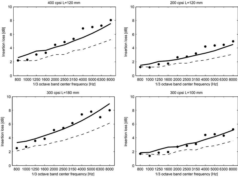
Figure 3.19: The simulated (lines) and measured (marks) insertion losses of the tested filters in the non-plane wave frequency range. The uncorrected simulation results (with the correction factor of  $\xi = 1.00$ ) are plotted with dashed lines and results with the correction factor of  $\xi = 1.48$  with solid lines. From Paper VI [42].
