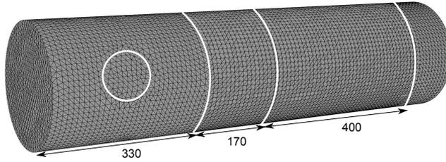
Figure 3.5: Finite element model of the one metre  $\varnothing=255$  mm test duct and the locations (mm) of the measurement cross-sections selected according to the low frequency plane wave decomposition criteria [3]. Both terminations are reflection-free, and this is modelled with infinite elements. The  $\varnothing=100$  mm circular region at the duct wall is the excitation area (“monopole”).
