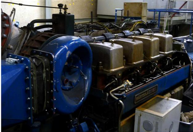
Figure 3.9: The test engine, Wärtsilä Vasa 4R32 in the VTT engine laboratory.
