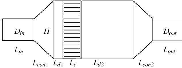
Figure 3.13: Schematic of the tested after-treatment device (see Paper V [40]). The main dimensions and the substrate (hatched area) properties are listed in Tables 3.3 and 3.4, respectively.
