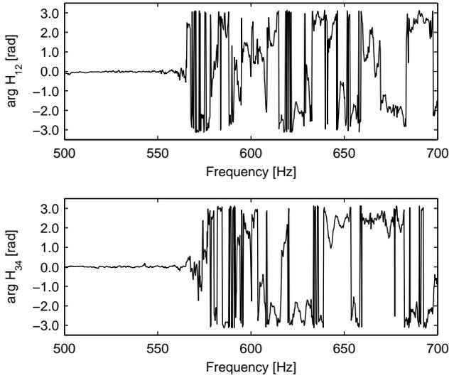
Figure 3.10: The measured phase shift between the opposite microphones, one-three above and two-four below. The phase of microphones one-three and two-four turns from in phase to out phase ( $\arg(H) \approx \pi$  rad) at frequencies of 568.5 Hz and 578.3 Hz respectively. Using these measured cut-on frequencies, the speed of sound can be determined, see Paper III [41].
