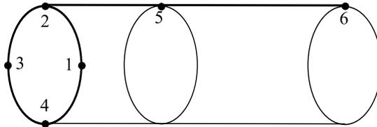
Figure 3.11: Pressure transducer configuration used in the exhaust pipe after the turbocharger. The axial and circumferential configurations consist of transducers 2-5-6 and 1-2-3-4 respectively, see Paper III [41].
