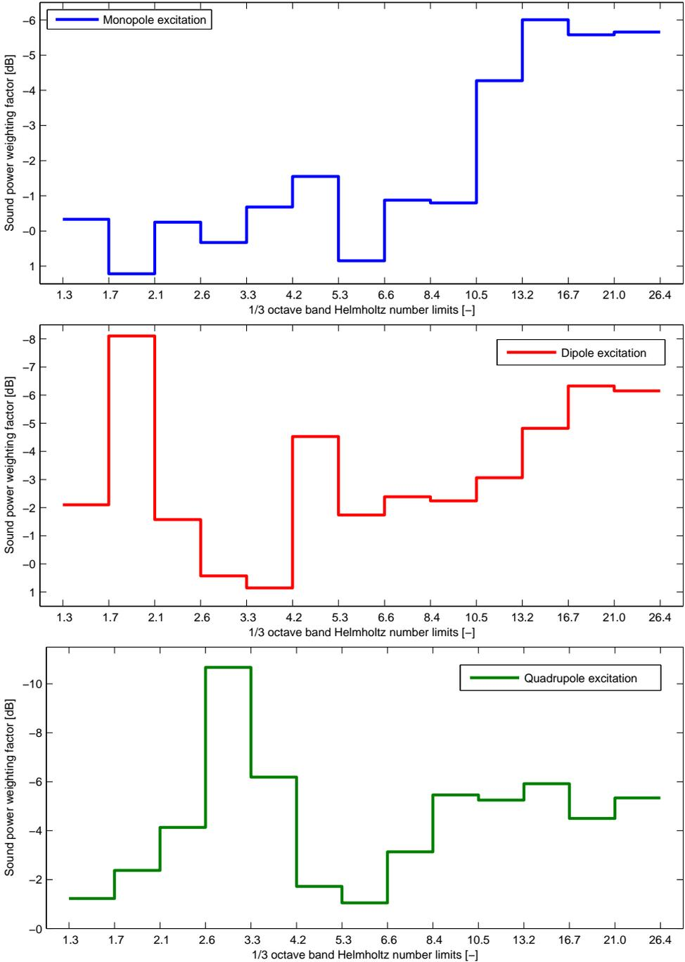
Figure 3.4: The experimentally derived 1/3 octave frequency band acoustic power weighting factors as a function of the 1/3 octave band Helmholtz number limits for monopole, dipole and quadrupole excitations.
