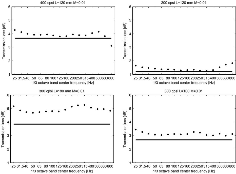
Figure 3.20: The simulated (lines) and measured (marks) transmission losses of the tested filters in the plane wave frequency range with  $M=0.01$ . From Paper VI [42].
