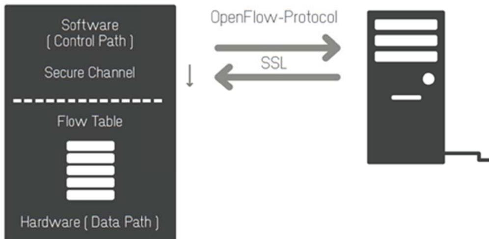
Figure 2-1: An OpenFlow-switch communicating with an SDN controller over a secure connection (SSL) via the OpenFlow protocol (a recreation from Figure 1 of [15])
