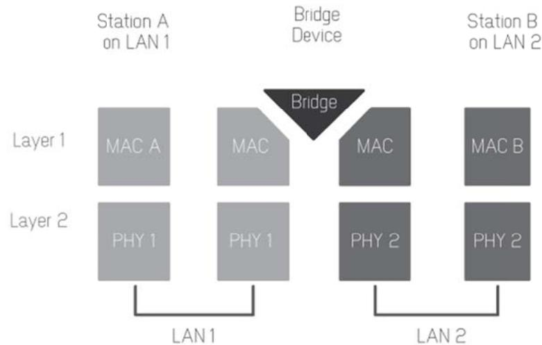
Figure 2-4: Bridging two LANs (or VLANs) via a shared bridge entity on layer 2
