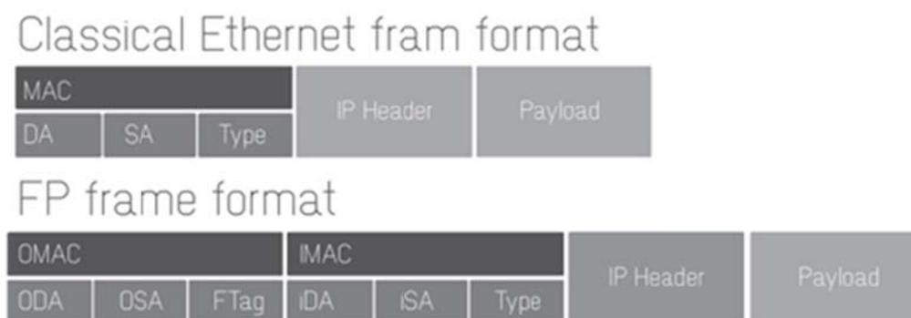
Figure 2-6: FabricPath header and its components
