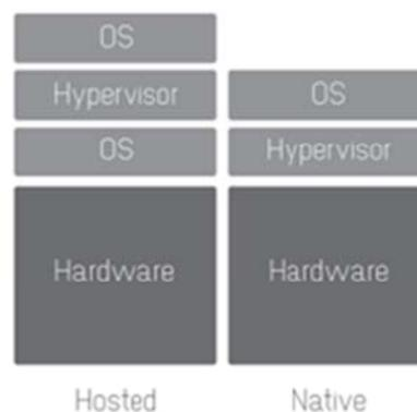
Figure 2-9: Alternative server virtualization stacks
