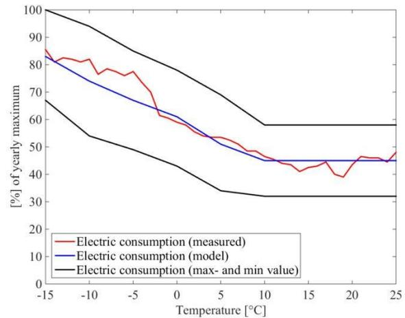
Fig. 3 Illustration of Smart Grid Gotland electricity consumption model as a function of temperature including comparison with the average of the measured electricity consumption at different temperatures
