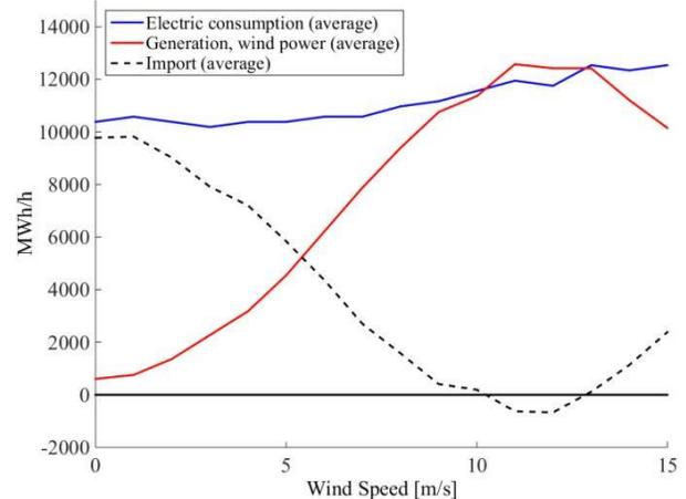
Fig. 4. Smart Grid Gotland's average electricity consumption, wind power generation and import as a function of as a function of wind speed
