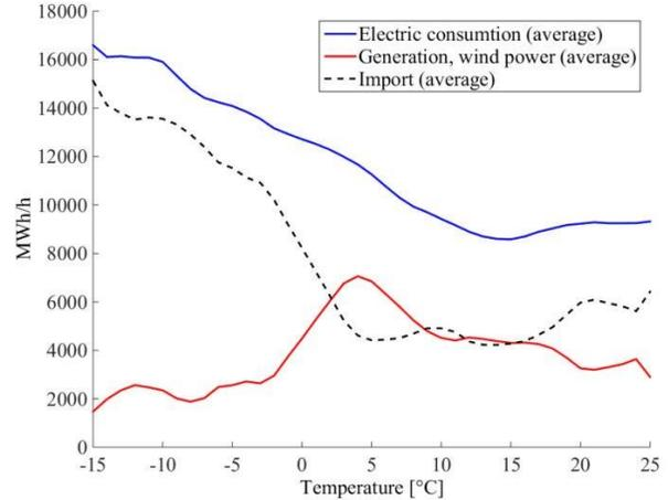
Fig. 2 Gotland's average electricity consumption, wind power generation and import as a function of outdoor temperature
