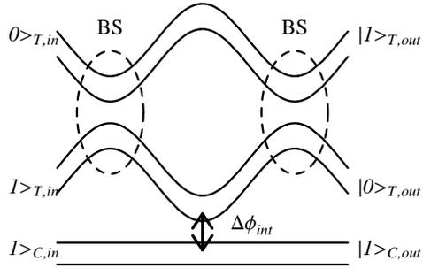
Figure 9: Schematic view of a controlled-NOT gate realised using an interferometer and a phase gate. The target qubit is incident in a superposition of the interferometer input modes. The control qubit is able to flip the target qubit as explained in the text.
