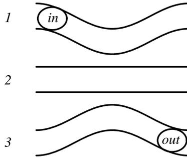
Figure 5: A single particle incident in channel 1 will exit in channel 3.
