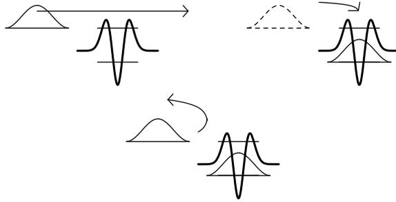
Figure 4: Schematic pictures of the gate operation. A wave packet with the correct energy will tunnel through the double barrier (upper left). Applying a suitable laser pulse, a particle can be trapped in the ground state (upper right). A second particle trying to pass will then be reflected (lower centre).
