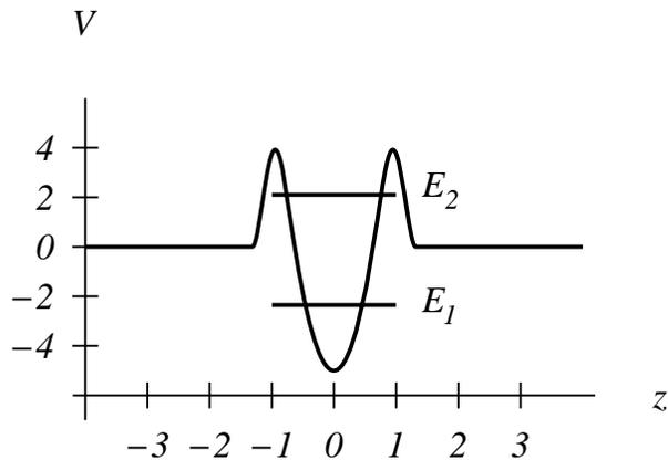
Figure 3: The gate potential  $V(z)$ . The particles are propagating in the  $z$  direction in the matter wave guide, confined in the  $x$  and  $y$  directions. The energies  $E_1$  of the bound ground state and  $E_2$  of the quasibound tunneling state are indicated with horizontal lines.
