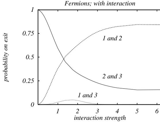
Figure 8: The probabilities, as functions of interaction strength, that two fermions, incident in channels 1 and 2, will exit at different combinations of output ports. Ideally, the probability for appearance in channels 1 and 2 should approach unity. The interaction strength is shown in units of  $V_{nn}/\Delta E$  as in figure 7.
