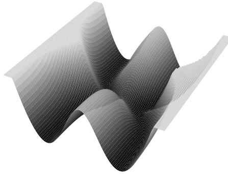
Figure 2: Atomic beam splitter potential. A beam splitter for atoms could be obtained by coupling two guides, in analogy with an optical coupler. The particle is allowed to tunnel between the guides where they approach each other.
