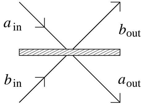
Figure 1: Schematic drawing of a beam splitter. The incoming modes  $a_{\text{in}}, b_{\text{in}}$  are piloted into the outgoing modes  $a_{\text{out}}, b_{\text{out}}$  according to the beam splitter relations.
