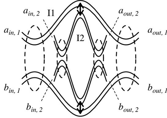
Figure 10: Bell-state analyser consisting of two coupled interferometers.
