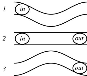
Figure 6: Two particles incident in channels 1 and 2 will exit in channels 2 and 3 supposing no particle-particle interaction is present.
