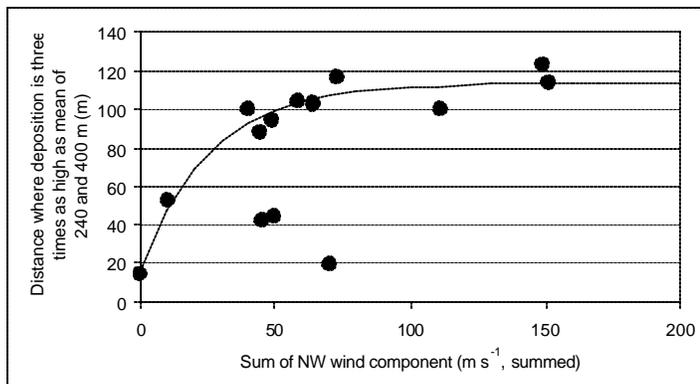
**Figure 11** The distance at which the amount of deposition of chloride was three times that measured at a distance well away from the road. The dashed curve is a hypothetical function describing the influence of the wind speed on the air-borne transport mechanism
