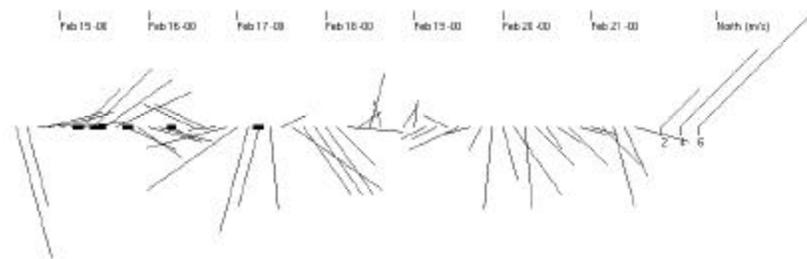
**Figure 18** *A sea weed diagram of the winds during investigation week 5 in the year 2000 investigation of bulk deposition pattern. The thin lines are vectors representing the three hour wind measurements (pointing in the downwind direction). In the far right end is a scale with the winds of 2, 4 and 6 m s<sup>-1</sup> pointing towards a true north direction. The black boxes are the time range, when the salting action has taken place.*
