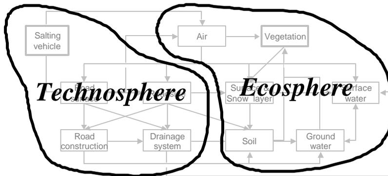
**Figure 15** *The box model of the physical system of de-icing salt (figure 3) as divided into the technosphere which is strongly influenced by the human activity of de-icing and the ecosphere, where the influence from de-icing is undesired.*
