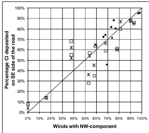
**Figure 10** Percentage of Cl deposited on the south-eastern side of the road as related to the percentage of winds with a NW-component. (? = 1998/99 12 m (n=13), \* = 1998/99 20 m (n=13), ? = 2000 14 m (n=9).
