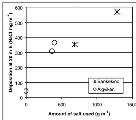
**Figure 8** *The relation of salt-use and deposition of salt at 20 m distance (data from Paper II)*
