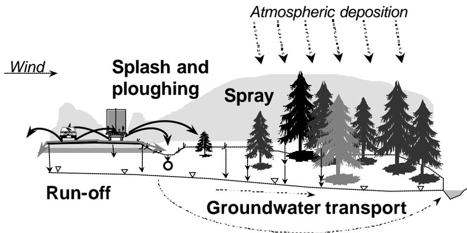
**Figure 2** *A conceptual model of the transport mechanisms and pathways from the road.*
