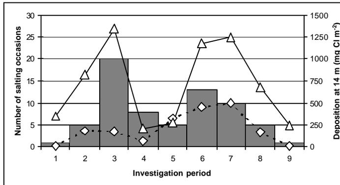
**Figure 9** *The number of salting occasions (bars) as compared to deposition of salt at 14 m distance (Paper III). Triangles represent deposition on the southeastern side of the road, and squares represent the deposition on the northwestern side of the road.*
