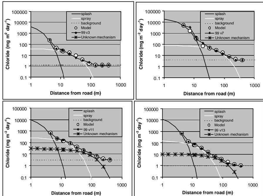
**Figure 17** *Examples of different deposition pattern from the 1998/-99 investigation. Data from Paper III is used to test the model of added splash, spray and background mechanisms. In the two upper pictures (week three and seven) the described model(Blomqvist, 1999) is sufficient, but in the two lower pictures (week 11 and 13) yet another mechanism needs to be added.*
