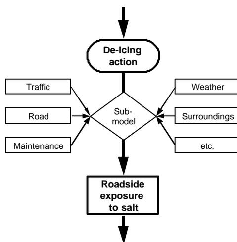
**Figure 16** *The segment of the DPSIR model between the de-icing action following the driving force (D) and the roadside exposure to salt could be described by a submodel that is a function of the characteristics of the traffic, road, maintenance, meteorological factors and physical factors.*
