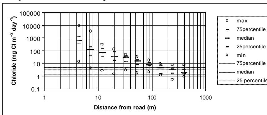
**Figure 7** Amount of chloride ( $\text{mg Cl}^2 \text{ day}^{-1}$ ) deposited in a profile perpendicular to the road, as compared to the background level (Paper III).
