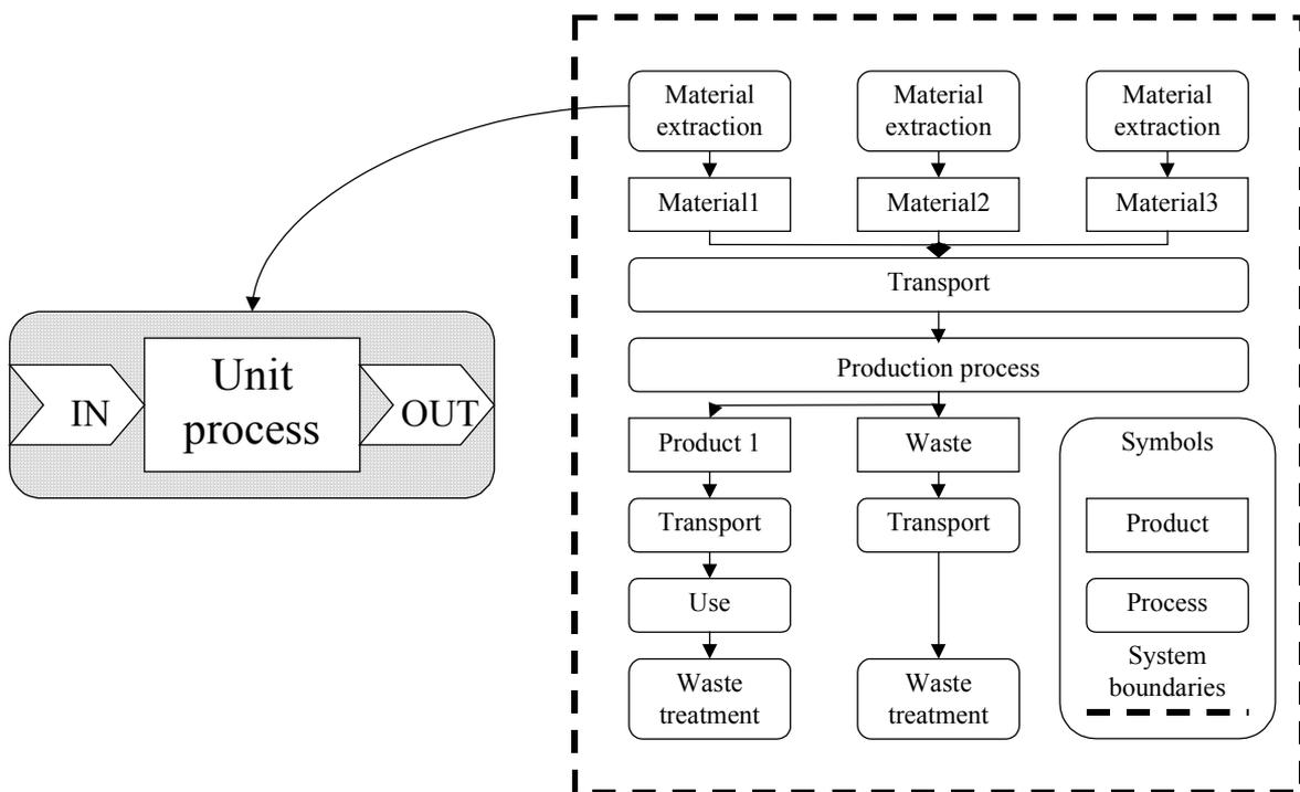
Figure 2. Process tree consisting of unit processes (Paulsen 1999a).
