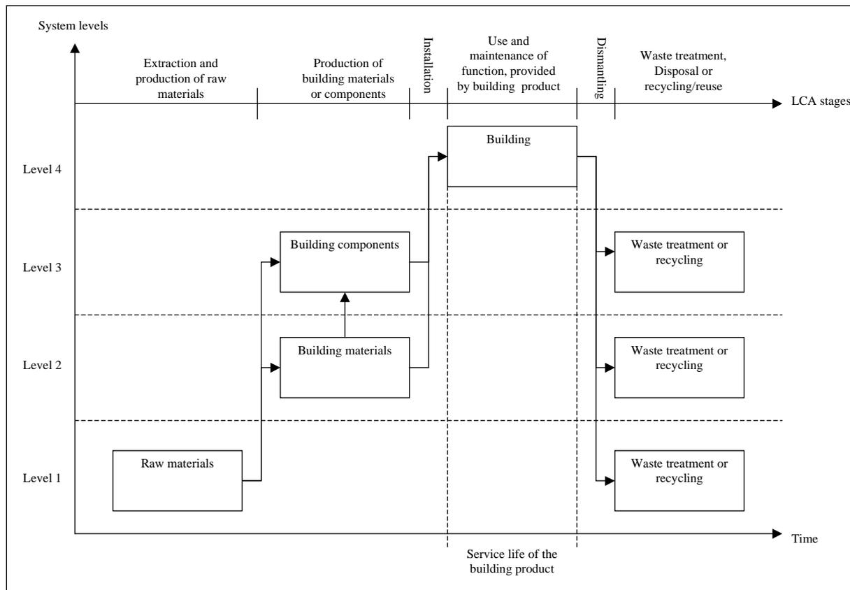
Figure 3.1 System levels in a building products life cycle (*Paper V*).
