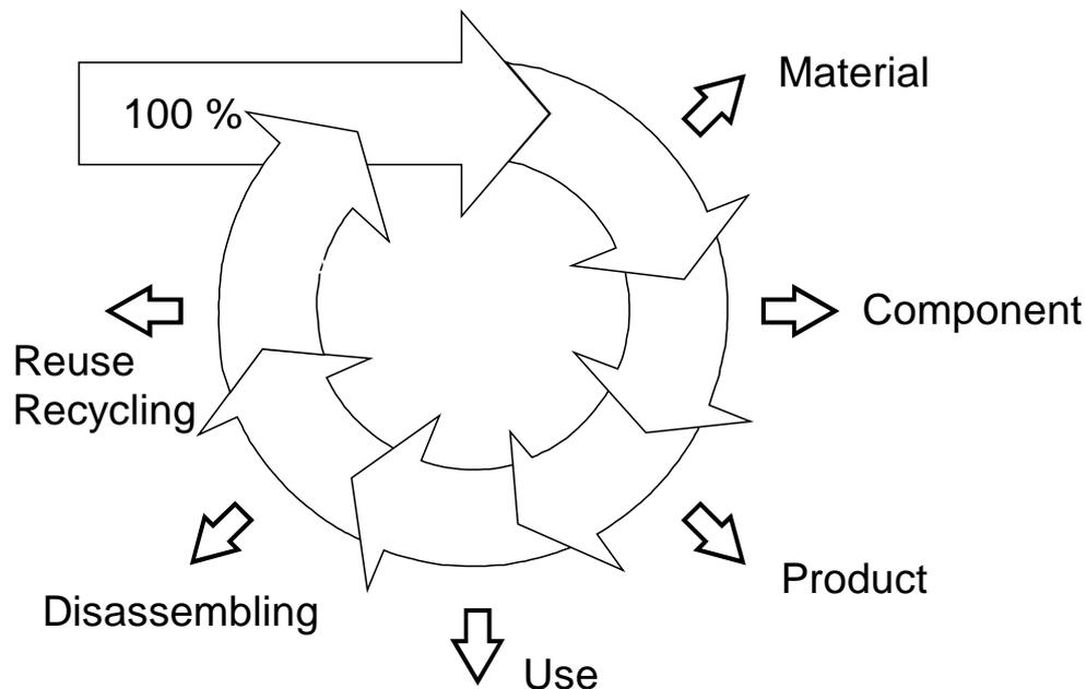
Figure 5.2 A schematic representation of the Yield, the circle, and losses due to different processes, the small arrows, during the life cycle for a product (**Paper I**).
