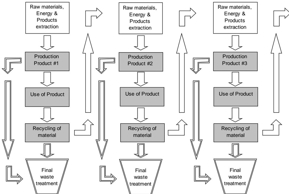
Figure 5.1 Cascade recycling system.
