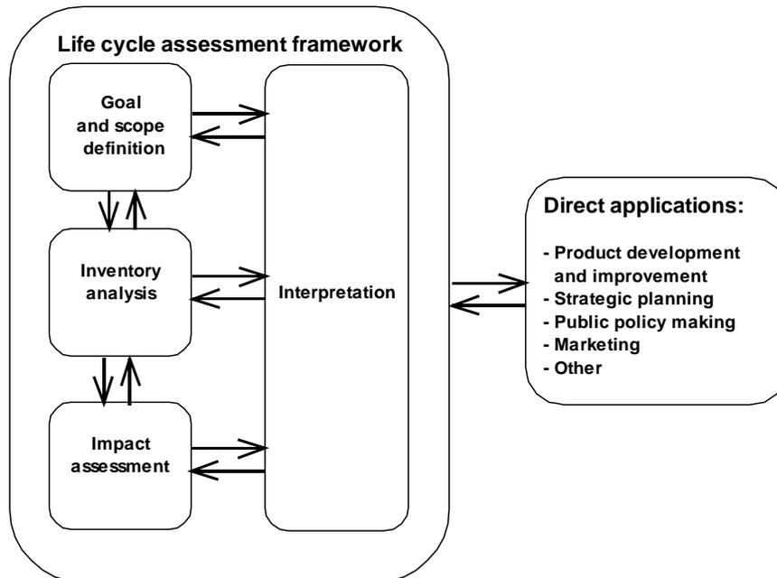
Figure 2.1 Phases of an LCA (ISO, 1997).
