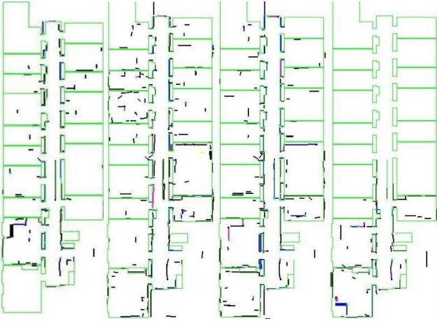
Fig. 3. This shows maps of our laboratory made with four different robots using the same configuration parameters for the EKF SLAM program. From left to right: a Performance PeopleBot, a Pioneer2DX, a PowerBot, and a custom built robot. The lighter lines are the hand made map shown for reference. The darker lines are the SLAM map. The building is 13 \times 39 m.
