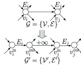
Fig. 5. The transformation of a network with vertex capacity to a network with edge capacity. In the new graph  $\mathcal{G}'$ , the capacity  $C_{ii} = E_i$ ,  $C_{ij} = +\infty$ ,  $C_{jj} = E_j$ .
