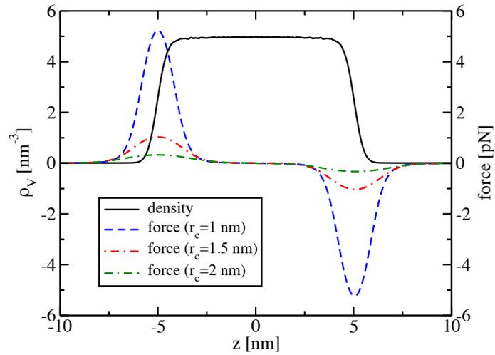
Figure 2: The density profile for a 10 nm slab of cyclohexane together with the added forces that compensate for the lack of long-range interactions.
