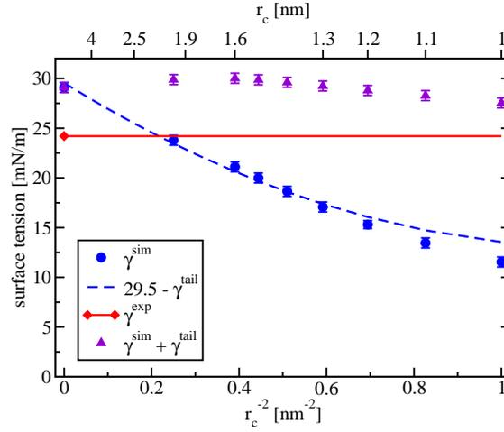
Figure 4: The surface tension of a cyclohexane surface with corrections added to the forces and to the surface tension. The experimental value is 24.2 mn/m at 300 K (13).
