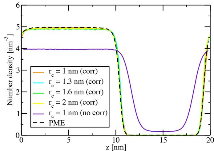
Figure 3: The density profile of a cyclohexane/vacuum-system with added corrections to the forces. The solid purple line without any corrections is for comparison.
