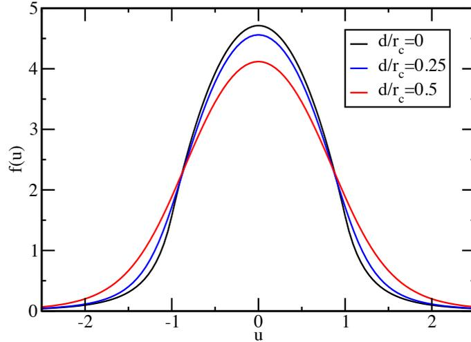
Figure 1: The dimensionless long range dispersion force perpendicular to a flat surface versus the dimensionless distance from the interface. The results are shown for a sharp surface and for a couple of  $d$ -values from a tanh-surface.
