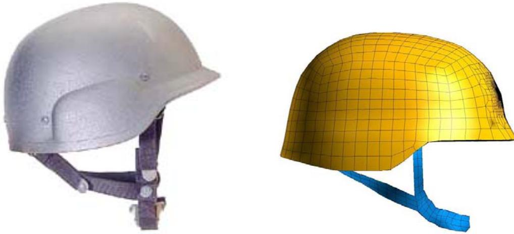
*Figure 10* A real ballistic helmet (left) and an FE model of a ballistic helmet (right).
