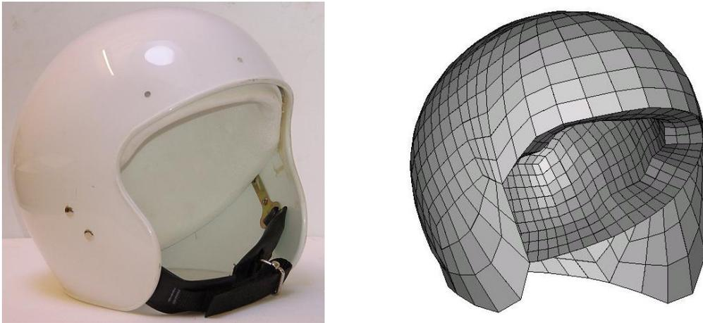
*Figure 9* The experimental helmet (left) and the FE model of the experimental helmet (right).
