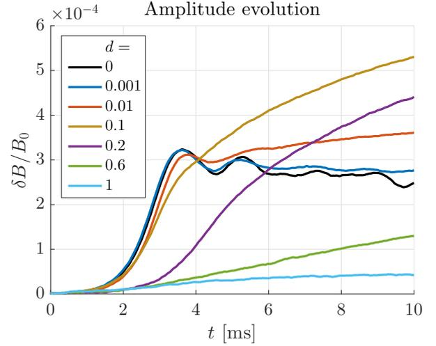
Figure 4. The evolution of the TAE amplitude for a set of proportionality constants  $d$  relative to the reference value of ICRH diffusion  $D_{\text{RF,ref}} = 0.32 \text{ MeV}^2/\text{s}$ .  $\delta B$  is the local maximum of the magnetic field around the  $q(\psi) = (5 + \frac{1}{2})/4$  surface, where  $q$  is the safety factor.
