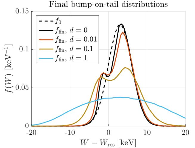
Figure 5. The initial bump-on-tail distribution (dashed curve) and final bump-on-tail distributions (solid curves, evaluated at  $t = 10 \text{ ms}$ ) for a subset of the cases presented in Fig. 4.
