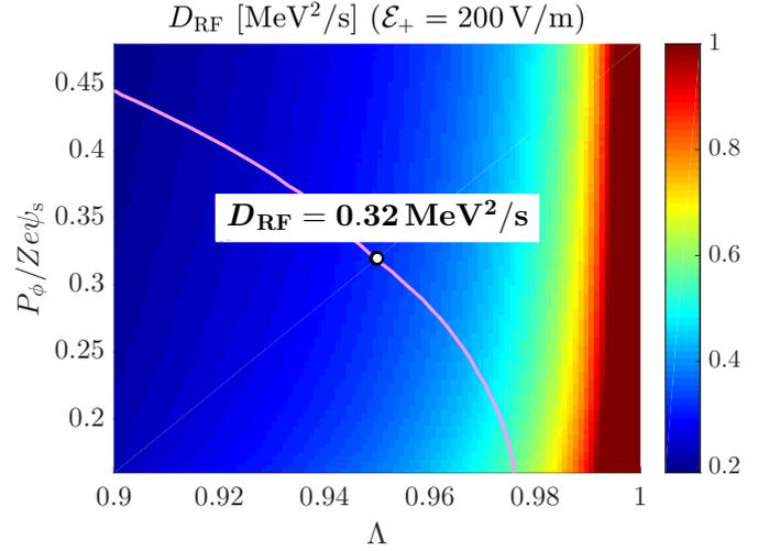
Figure 3. The ICRH diffusion coefficient of eq. (10) at  $\mu = 300 \text{ keV/T}$ . The colour scale of  $D_{\text{RF}}$  has an upper bound at  $1 \text{ MeV}^2/\text{s}$ , although the diffusion coefficient has far larger values close to the singularity at  $\Lambda = 1$ . The white dot shows the location of the reference point, where the constant value of  $D_{\text{RF}}$  used in the simulations is evaluated.
