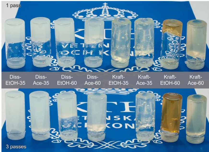
Figure 10. Nanocellulose oxalate after microfluidization at approximately 1.5 wt. %. The samples were homogenized with one pass through the microfluidizer (top) and three passes (bottom).
