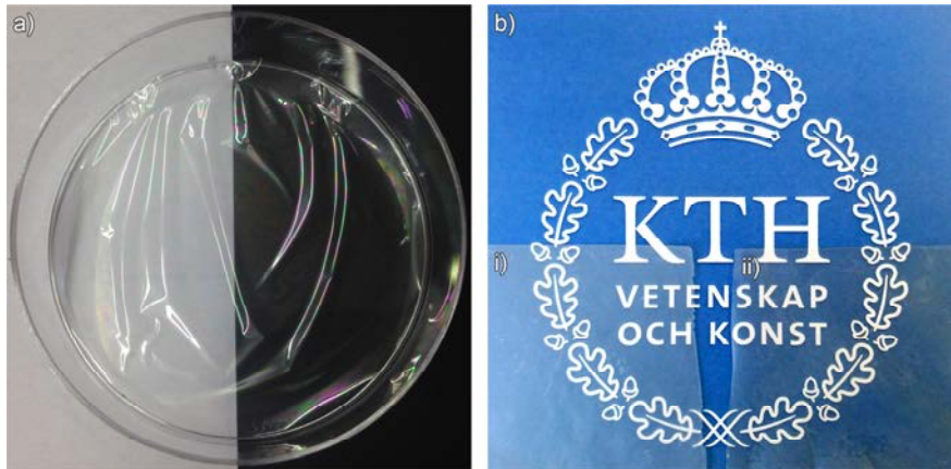
Figure 15. Films from nanocellulose oxalate, a) NDISS-THF-30 prepared by solvent casting, b) i) NKRAFT-ACE-35 with 5 passes and ii) NDISS-ACE-35 with 5 passes prepared through filtration over a membrane.
