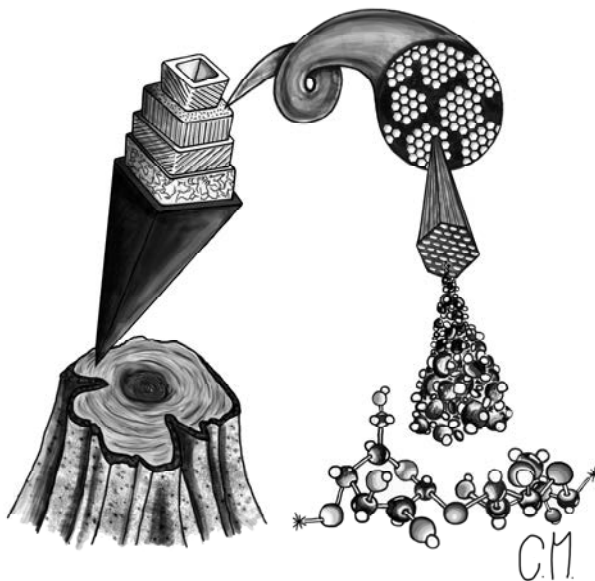
Figure 1. The hierarchical structure of wood ranging from cellobiose, the repeating unit in cellulose, to the elementary fibril, fibril aggregate, wood fibre and tree trunk. (© Carl Moser)
