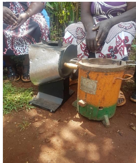
Figure 4.6: comparing the heights of the MiG|BioCooker (left) and Gastov (right)
