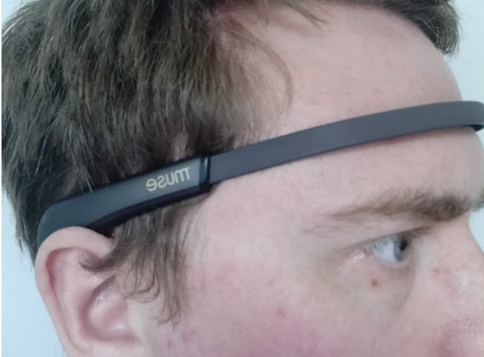
Figure A.7: The Muse 2 Brain Sensing Headband (Muse) in use. A reference electrode is positioned in the middle of the forehead (Fpz position), between two active electrodes (AF7 and AF8 positions). One electrode is position behind each ear (TP9 and TP10).
