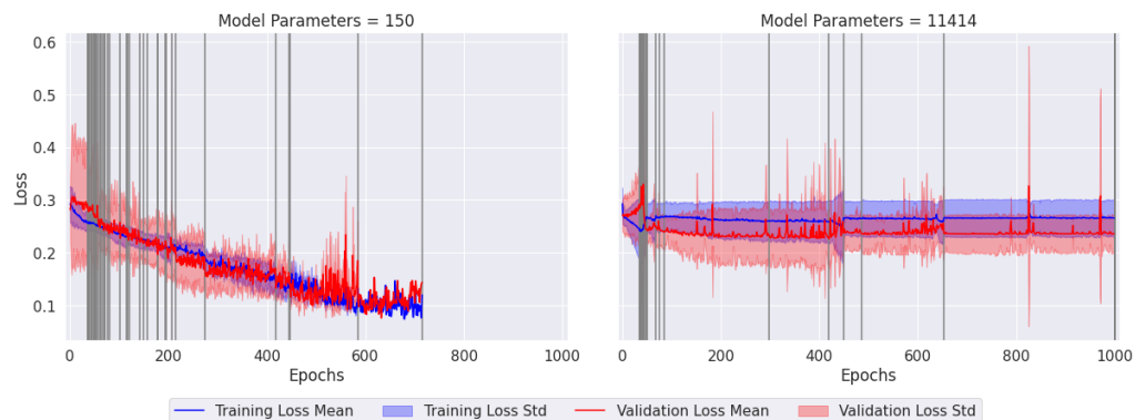
Figure 4.4. Loss curves for small and large configuration in Vanilla CNN Experiment 1. The loss for each epoch is averaged over all runs and folds of the configuration that have not been stopped. The mean and standard deviation are shown. A vertical grey line shows when the training for one fold was stopped.
