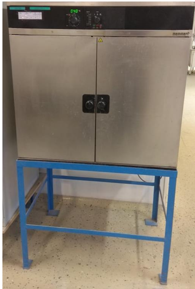
Figure 5. The ventilated oven that was used for the water content determination test
