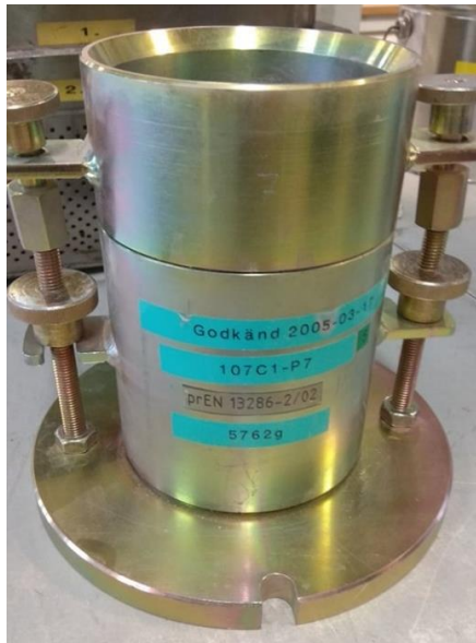
Figure 6. The cylindrical mould used for the modified Proctor compaction test
