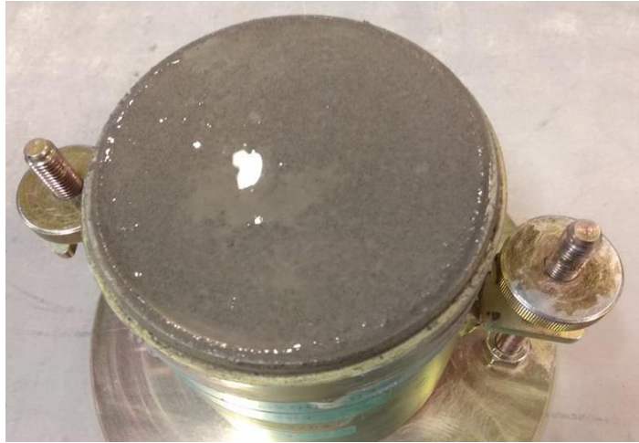
Figure 13. Self-draining mixture (sample No. 7) during compaction of material 0/4 for moisture content 12%
