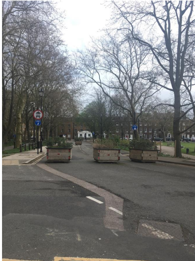
Figure A7.2. The figure shows modal filters by the entrance to the area Highbury West in Islington. Picture taken by Greta Gustafsson.
