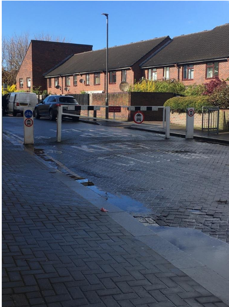
Figure A7.4. The figure shows an example of the modal filters by the entrance to the LTN in Wandsworth that is part of this study. Picture taken by Greta Gustafsson.
