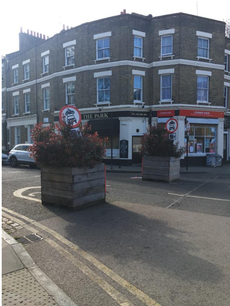
Figure A7.4. The figure shows an example of modal filters in Hackney (not a borough that is part of the study). Picture taken by Greta Gustafsson.
