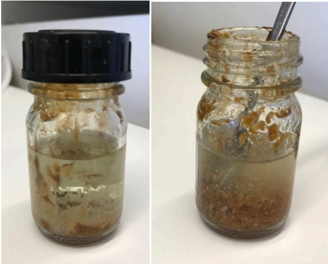
FIGURE 12. MTP, AFTER 4 WEEKS OF STORAGE AT 40°C, BEFORE STIRRING (TO THE LEFT) AND AFTER STIRRING (TO THE RIGHT).
