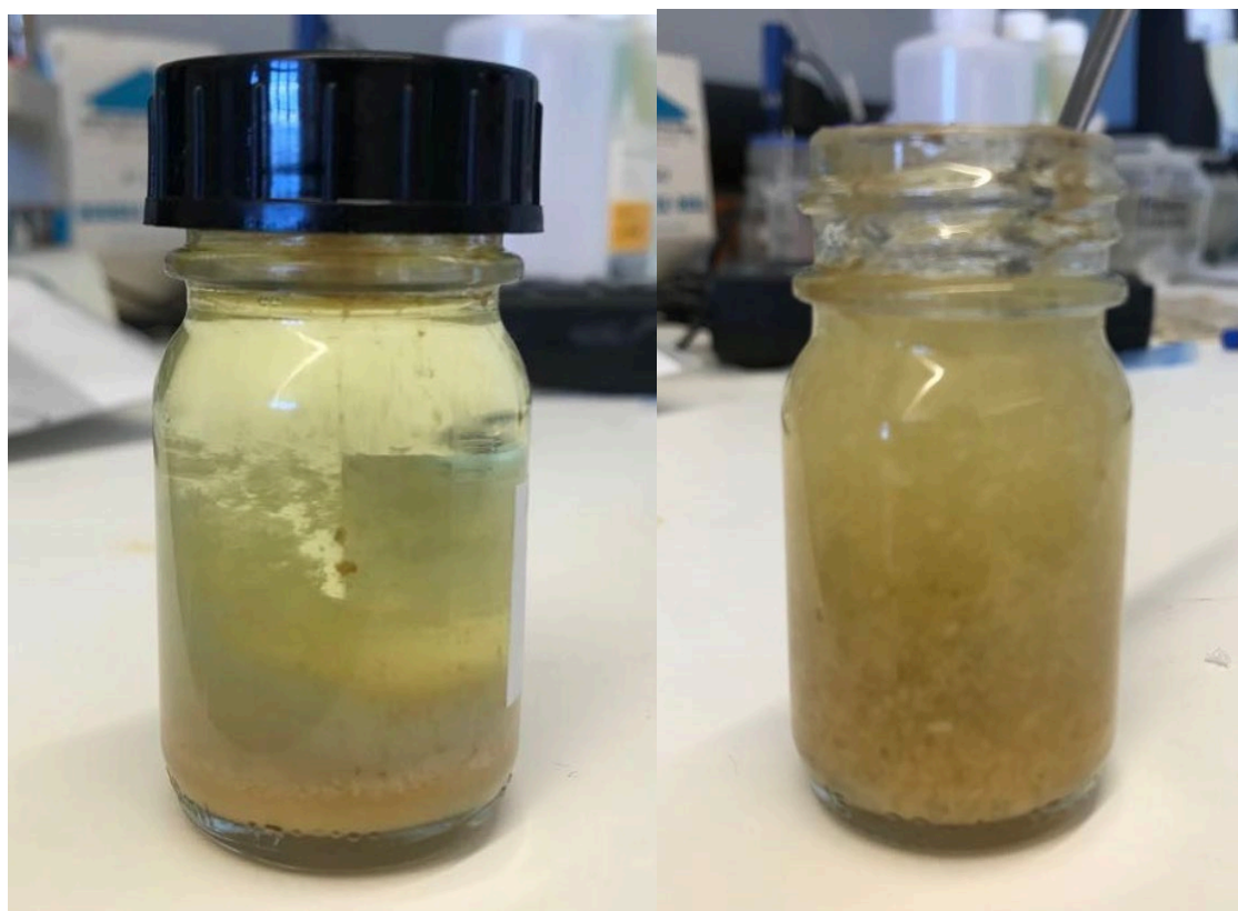
FIGURE 11. OTP, AFTER 4 WEEKS OF STORAGE AT 40°C, BEFORE STIRRING (TO THE LEFT) AND AFTER STIRRING (TO THE RIGHT).
